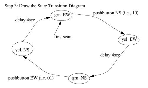
Figure 12.8 A Traffic Light State Diagram
