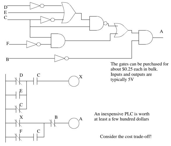
*Figure 6.8* A Boolean Equation and Derived Circuit and Ladder Logic
