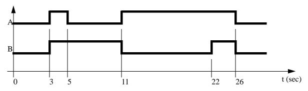
3. Use the timing diagram below to design ladder logic. The sequence should start when input *X* turns on. X may only be on momentarily, but the sequence should execute anyway.
