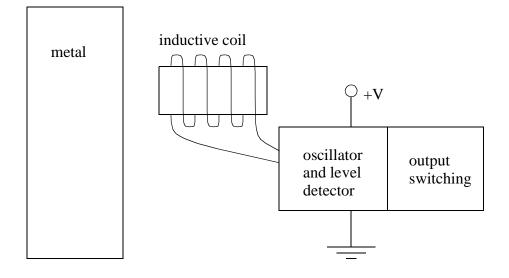
Note: these work by setting up a high frequency field. If a target nears the field will induce eddy currents. These currents consume power because of resistance, so energy is in the field is lost, and the signal amplitude decreases. The detector examines filed magnitude to determine when it has decreased enough to switch.
