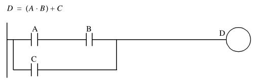
Figure 6.15 Sample Solution for Logic Case Study A
