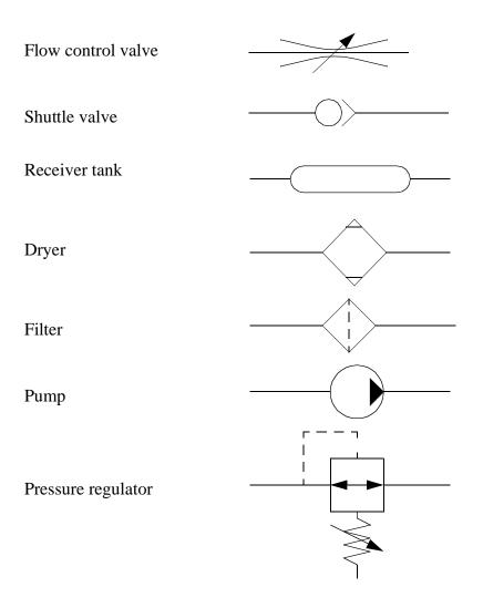
*Figure 5.7* Pneumatics Components
