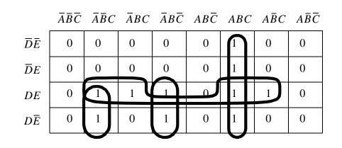
$X = ABC + D(\overline{A}\overline{B}C + \overline{A}B\overline{C} + EC)$
