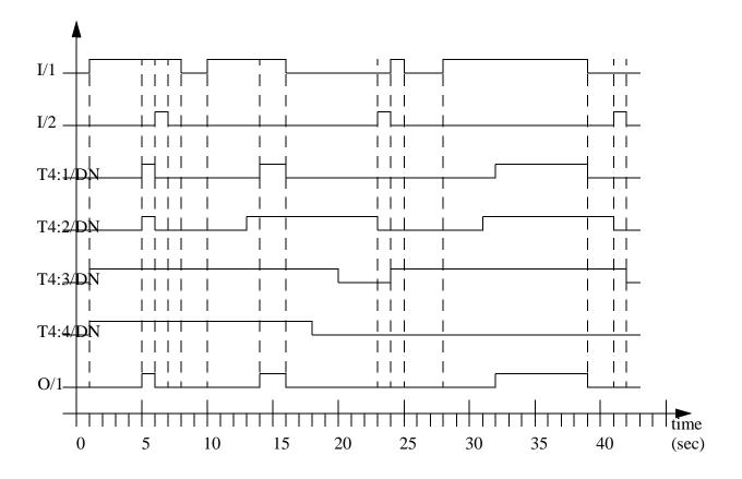
*Figure 9.12* A Timing Diagram for Figure 9.11
