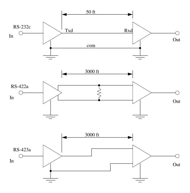
*Figure 27.2* Serial Data Standards
