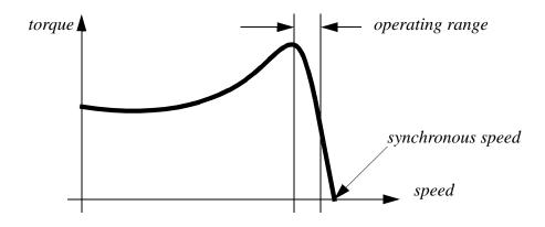
Figure 24.10 Torque Speed Curve for an Induction Motor
