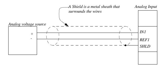
Figure 23.32 Cable Shielding
