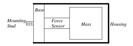
Figure 23.12 A Cross Section of an Accelerometer
