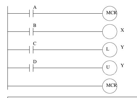
Note: If a normal input is used inside an MCR block it will be forced off. If the output is also used in other MCR blocks the last one will be forced off. The MCR is designed to fully stop an entire section of ladder logic, and is best used this way in ladder logic designs.
