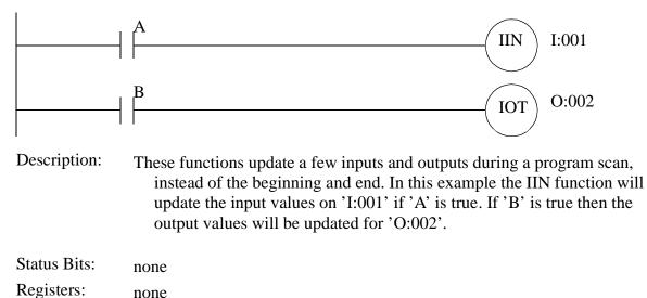
IIN, IOT - Immediate INput, Immediate OuTput
