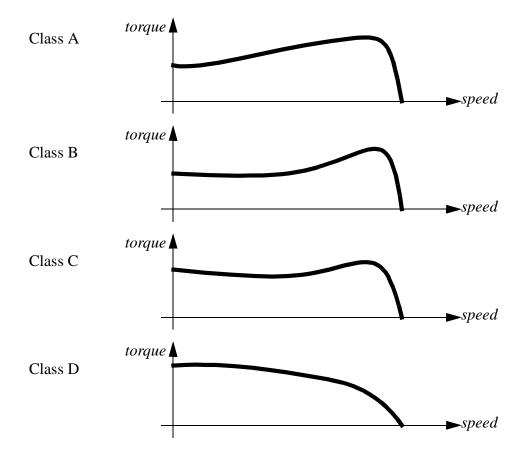
Figure 24.11 NEMA Squirrel Cage Torque Speed Curves
