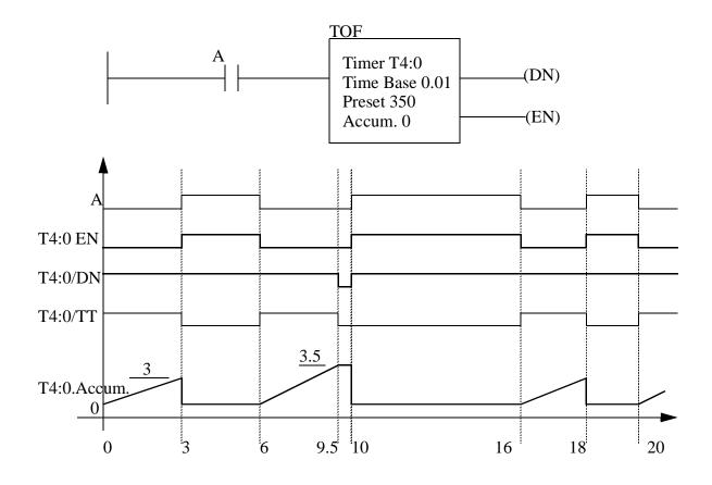
Figure 9.10 An Allen Bradley Off-Delay Timer
