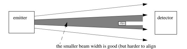
Figure 4.17 The Relationship Between Beam Width and Object Size
