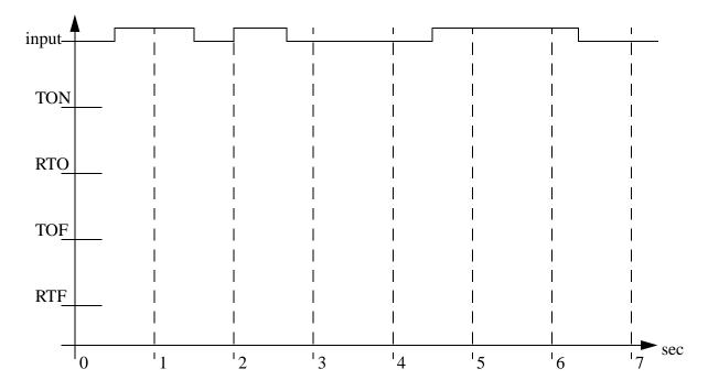
9. Given the following timing diagram, draw the done bits for all four fundamental timer types. Assume all start with an accumulated value of zero, and have a preset of 1.5 seconds.
