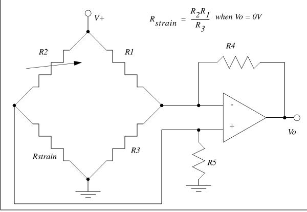
Figure 23.18 Measuring Strain with a Wheatstone Bridge
