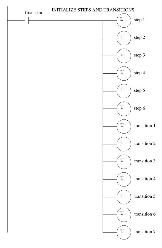
Figure 20.5 SFC Implemented in Ladder Logic
