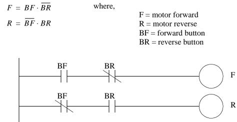
*Figure 6.18* Motor Forward, Reverse Case Study
