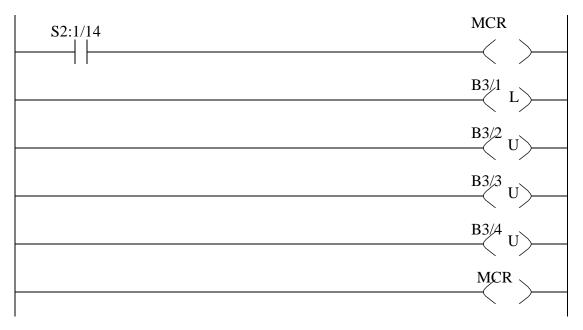
Figure 12.10 Ladder Logic to Initialize Traffic Light Controller
