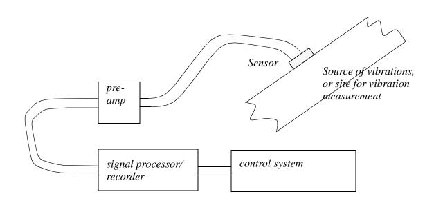
*Figure 23.15* Typical Connection for Accelerometers
