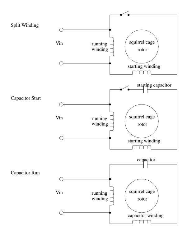
Figure 24.12 Single Phase Motor Configurations
