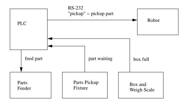
Figure 28.16 Box Loading System
