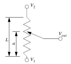
$$V_{out} = V_1 + (V_2 - V_1) \left(\frac{a}{I}\right)$$
