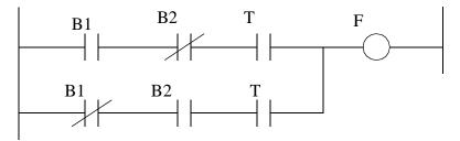
*Figure 6.6* Alternate Ladder Logic
