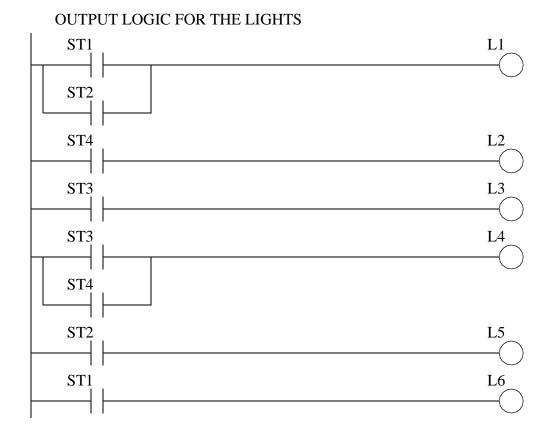
Figure 12.23 Ladder Logic for the State Equations
