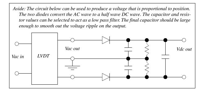
Figure 23.9 A Simple Signal Conditioner for an LVDT
