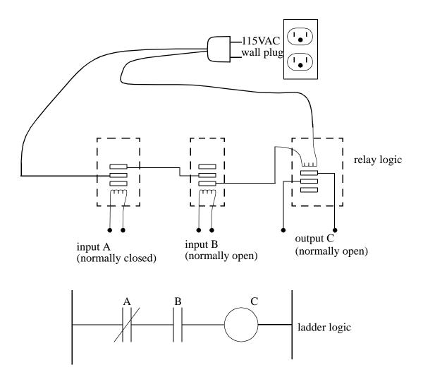
*Figure 2.2* A Simple Relay Controller
