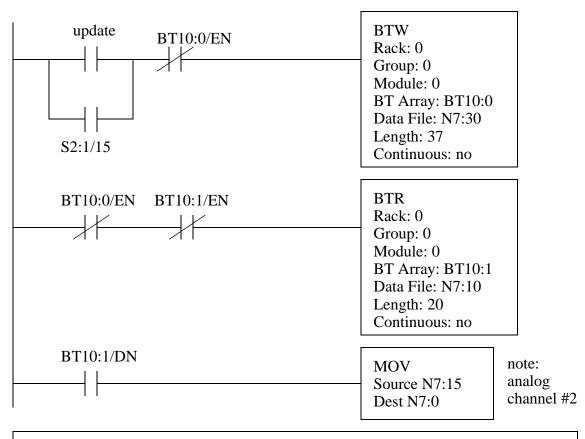
Note: The basic operation is that the BTW will send the control block to the input card. The inputs are used because the BTR and BTW commands may take longer than one scan.
