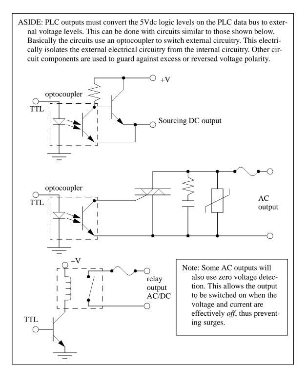
*Figure 3.4* Aside: PLC Output Circuits
