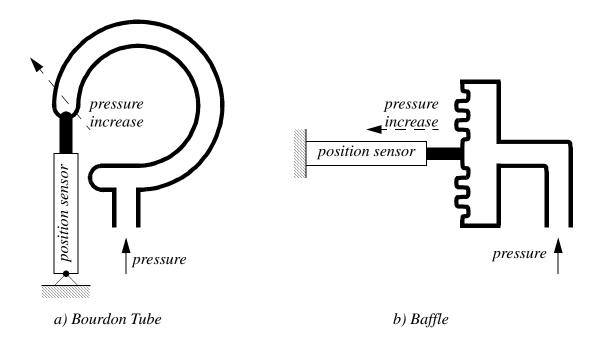
Figure 23.22 Pressure Transducers
