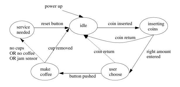
*Figure 12.3* State Diagram for a Coffee Machine
