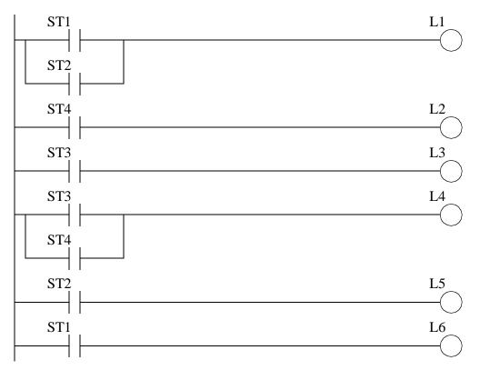
*Figure 12.30* Ladder Logic for the State-Transition Equations
