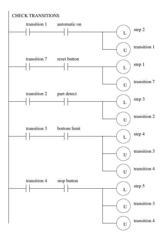
Figure 20.6 SFC Implemented in Ladder Logic
