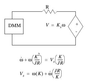
When the motor shaft is turned by another torque source a voltage is generated that is proportional to the angular velocity. This is the reverse emf. A dmm, or other high impedance instrument can be used to measure this, thus minizing the loses in resistor R. encoders cost more but can have higher resolutions. Potentiometers have limited ranges of motion
