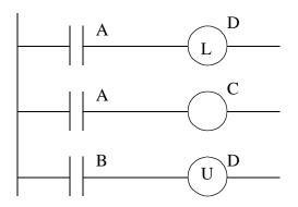
*Figure 9.2* A Ladder Logic Latch
