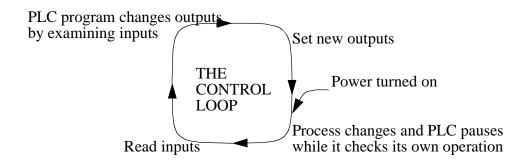
*Figure 2.10* The Scan Cycle of a PLC
