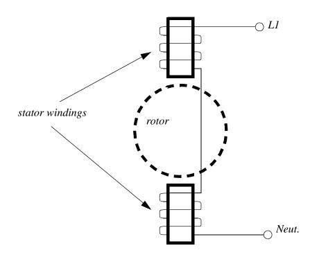
*Figure 24.7* A 2 Pole Single Phase AC Motor
