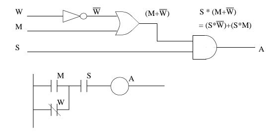
Figure 6.22 The Simplest Circuit and Ladder Diagram
