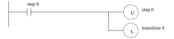
Figure 20.9 SFC Implemented in Ladder Logic
