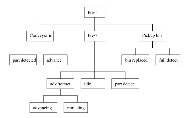
*Figure 32.5* Functional Diagram for Press Control
