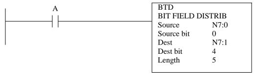
Description: This function will copy the bits starting at N7:0/0 to N7:1/4 for a length of 5 bits.
