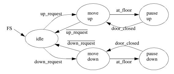
10. Write ladder logic for the state diagram below a) using an equation based method. b) without
