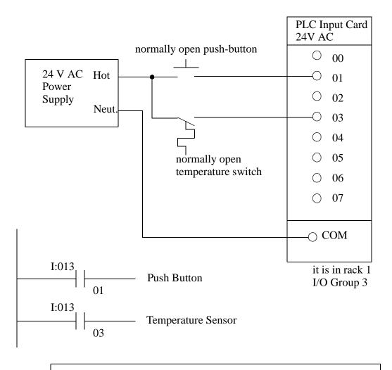
Note: inputs are normally high impedance. This means that they will use very little current.
