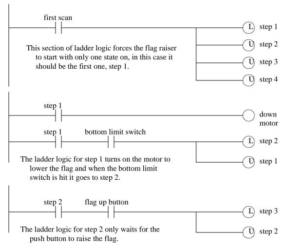
Figure 10.2 A Process Sequence Bit Design Example
