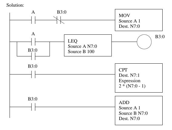
Figure 15.26 A Series Calculation Example
