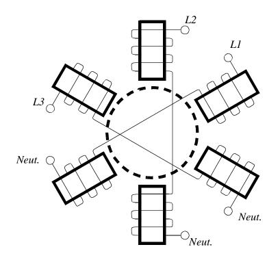
*Figure 24.8* A 6 Pole 3-Phase AC Motor
