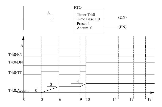
*Figure 9.9* An Allen Bradley Retentive On-Delay Timer
