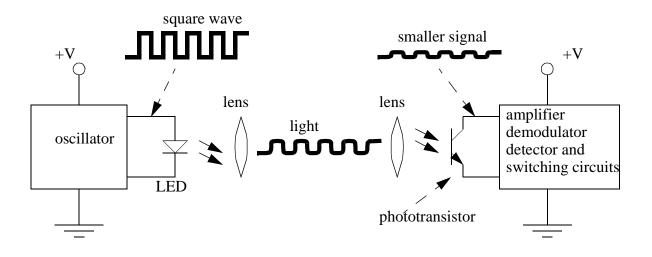
*Figure 4.11* A Basic Optical Sensor
