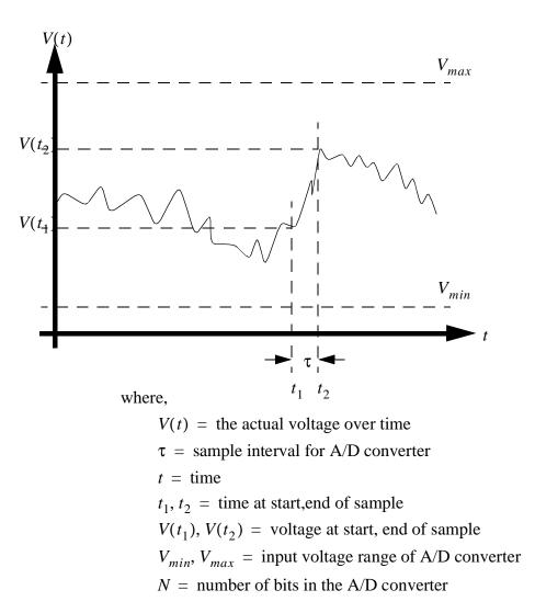
*Figure 22.3* Parameters for an A/D Conversion
