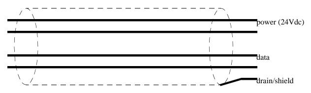
Thick trunk - carries up to 8A for power up to 500m Thin trunk - up to 3A for power up to 100m
