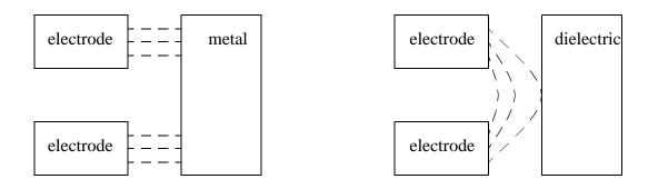
*Figure 4.24* Dielectrics and Metals Increase the Capacitance
