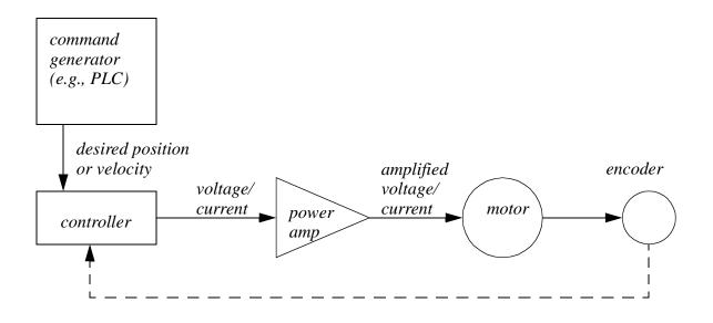
Figure 24.1 A Typical Feedback Motor Controller
