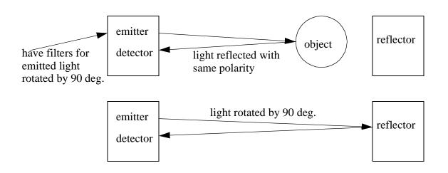
Figure 4.14 Polarized Light in Retroreflective Sensors
