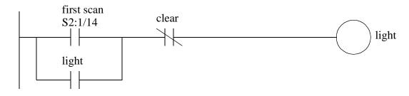
*Figure 8.6* An program that checks for the first scan of the PLC
