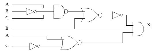
The circuit is converted to a Boolean equation and simplified. The most nested terms in the equation are on the left hand side of the diagram.
