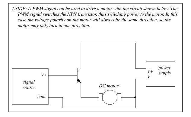
Figure 24.5 PWM Unidirectional Motor Control Circuit
