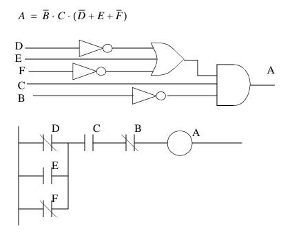
*Figure 6.9* The Simplified Form of the Example
