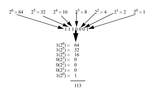
*Figure 13.3* Conversion of a Binary Number to a Decimal Number
