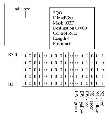
*Figure 16.8* A Sequencer For Traffic Light Control
