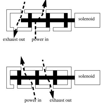
Figure 5.2 A Solenoid Controlled 5 Ported, 4 Way 2 Position Valve
