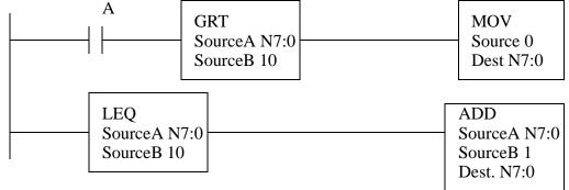
Figure 15.25 A Simple Comparison Example
