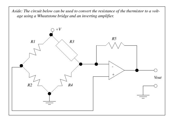
Figure 23.30 Thermistor Signal Conditioning Circuit
