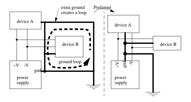
Figure 31.9 Eliminating Ground Loops
