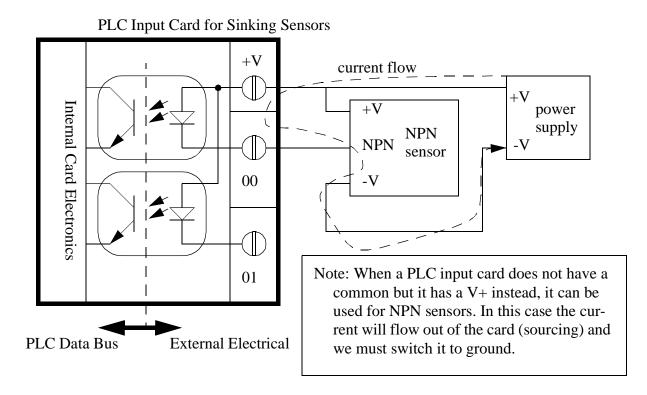
ASIDE: This card is shown with 2 optocouplers (one for each output). Inside these devices the is an LED and a phototransistor, but no electrical connection. These devices are used to isolate two different electrical systems. In this case they protect the 5V digital levels of the PLC computer from the various external voltages and currents.
