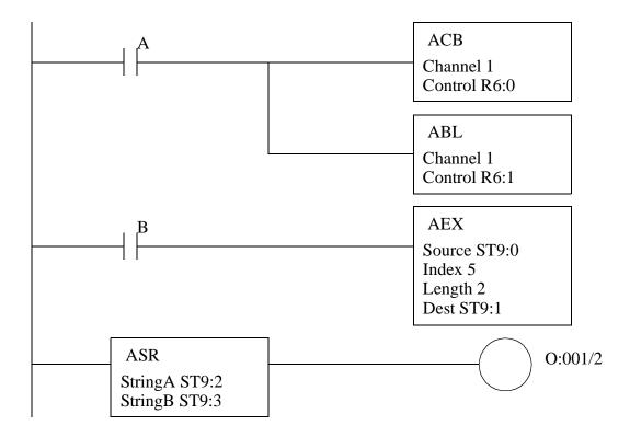
Figure 27.11 String Manipulation Functions
