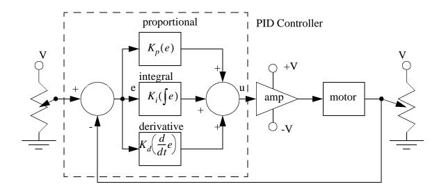
Figure 25.14 A PID Control System
