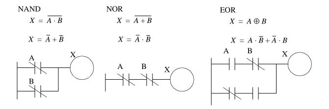
Figure 6.12 Conversion of Complex Logic Functions
