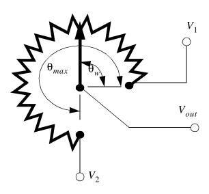
$$V_{out} = (V_2 - V_1) \left(\frac{\theta_w}{\theta_{max}}\right) + V_1$$
