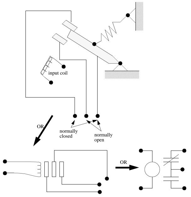
*Figure 2.1* Simple Relay Layouts and Schematics
