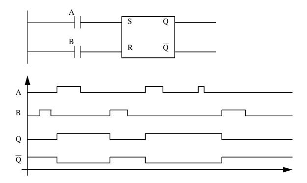
*Figure 9.6* Flip-Flops for Latching Values
