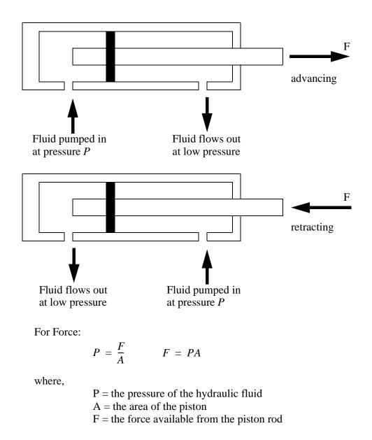
*Figure 5.4* A Cross Section of a Hydraulic Cylinder
