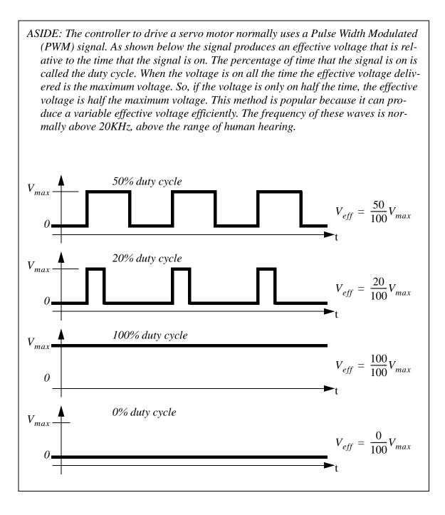
*Figure 24.4* Pulse Width Modulation (PWM) For Control
