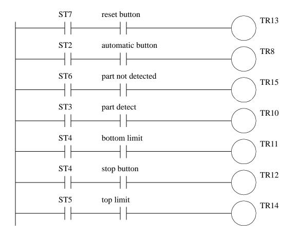
Figure 20.12 Ladder logic for transitions
