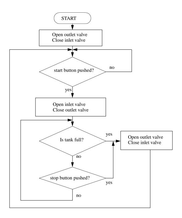
*Figure 11.2* A Flowchart for a Tank Filler
