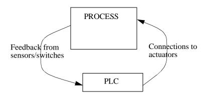
*Figure 2.9* The Separation of Controller and Process
