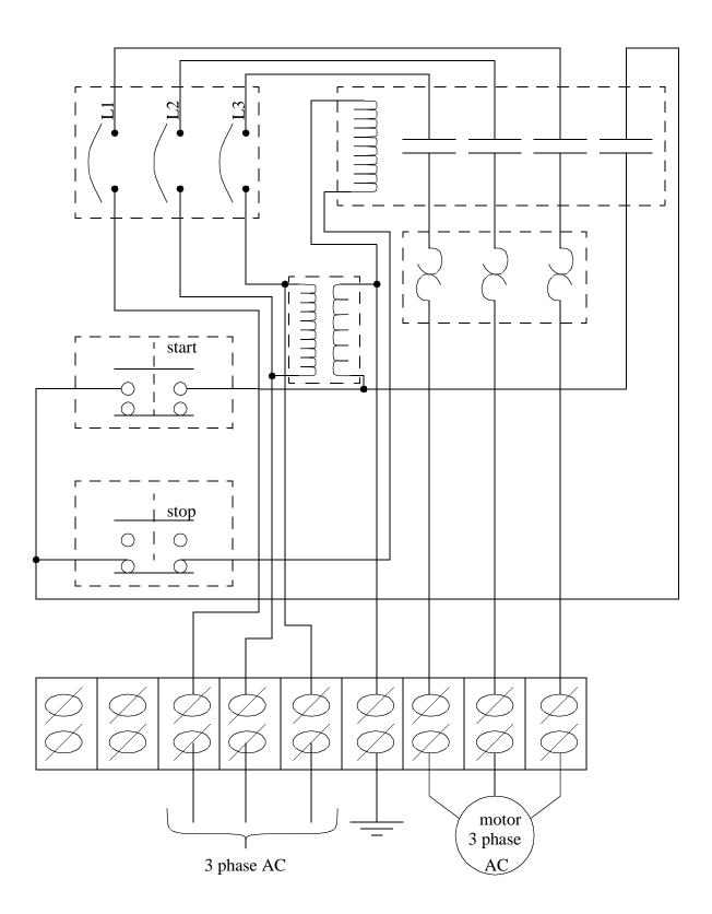
*Figure 31.3* Final Panel Wiring
