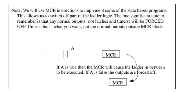
*Figure 11.4* The MCR Function
