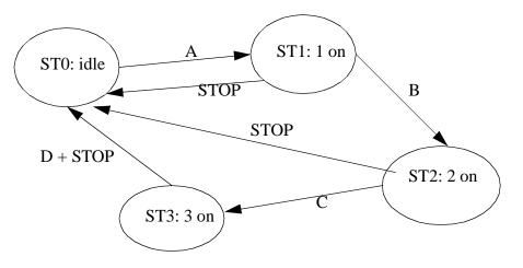
4. Convert the following state diagram to ladder logic using the delayed update method.
