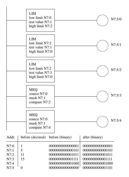
Figure 15.19 Complex Comparison Functions
