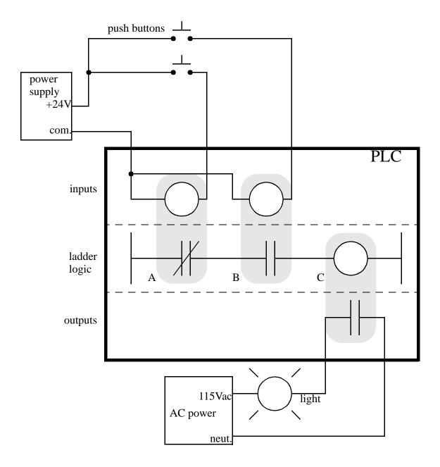
*Figure 2.3* A PLC Illustrated With Relays
