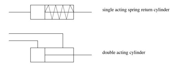
*Figure 5.5* Schematic Symbols for Cylinders
