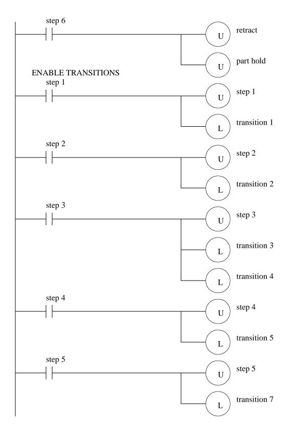
Figure 20.8 SFC Implemented in Ladder Logic
