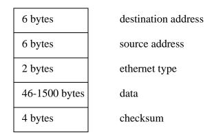
Figure 28.11 Ethernet Version II Frame
