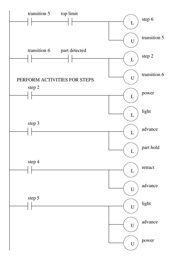
Figure 20.7 SFC Implemented in Ladder Logic
