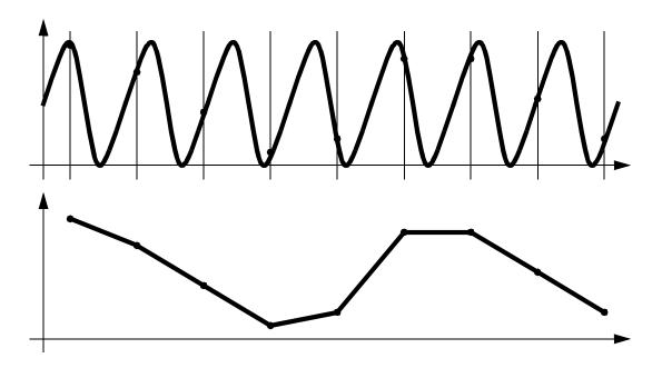
Figure 22.6 Low Sampling Frequencies Cause Aliasing
