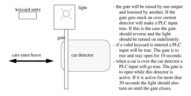
14. Use a state diagram to design a parking gate controller.
