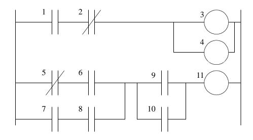
*Figure 8.4* Ladder Logic Execution Sequence
