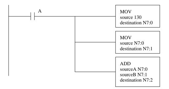
Figure 14.11 An Example of Ladder Logic Functions
