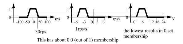
4. If  $v_{error}$  is ZE and  $d_{dt}v_{error}$  is SN then  $V_{motor}$  is SN.
