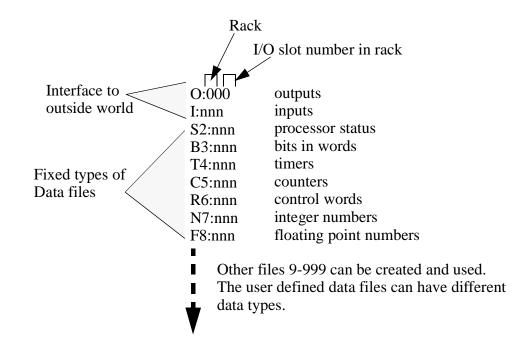
*Figure 14.2* Data Files for an Allen Bradley PLC-5
