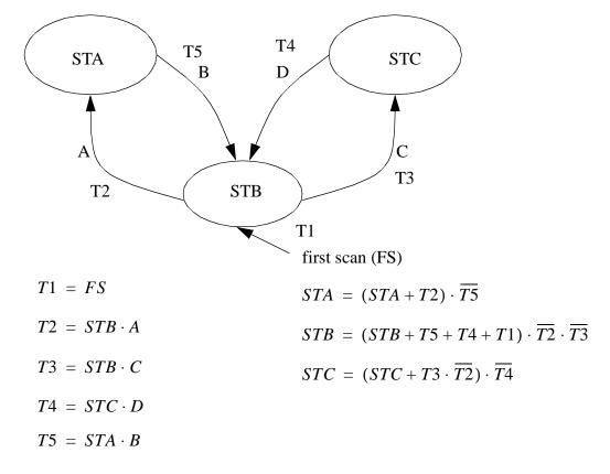
6. Implement the State-Transition equations.in the figure below with ladder logic.
