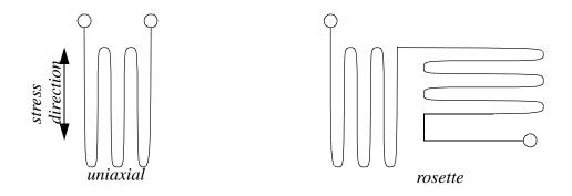
Figure 23.19 Wire Arrangements in Strain Gages
