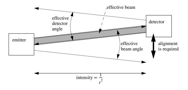
*Figure 4.16* Beam Divergence and Alignment
