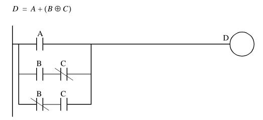
*Figure 6.16* Sample Solution for Logic Case Study B
