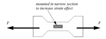
Figure 23.20 Using a Narrow to Increase Strain
