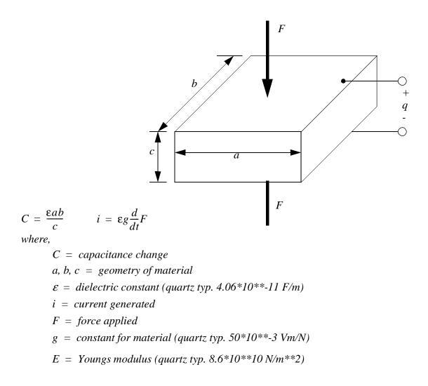
Figure 23.21 The Piezoelectric Effect
