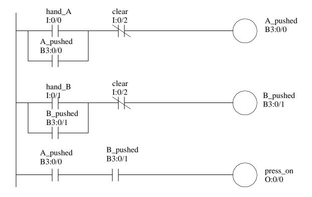
*Figure 9.20* An example using bit memory
