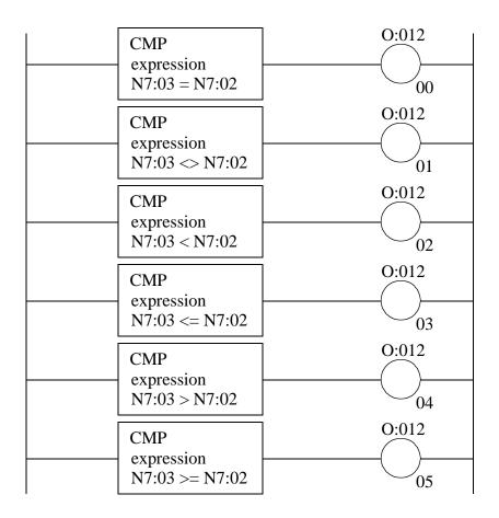
Figure 15.17 Equivalent Statements Using CMP Statements
