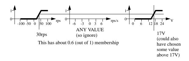
1. If  $v_{error}$  is LP and  $d/_{dt}v_{error}$  is any then  $V_{motor}$  is LP.
