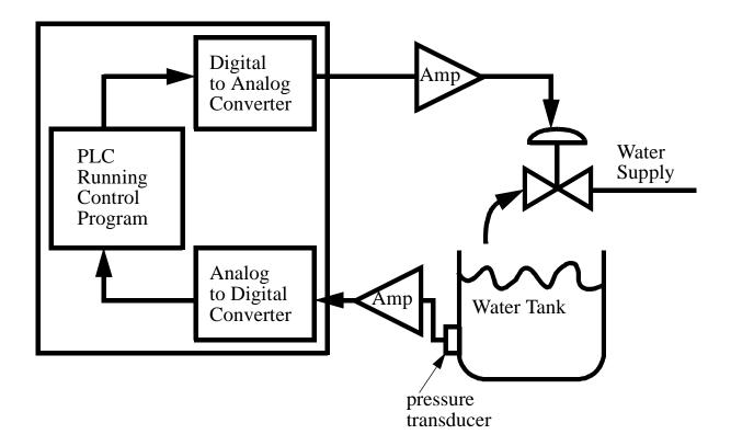
Figure 25.19 Water Tank Level Controller
