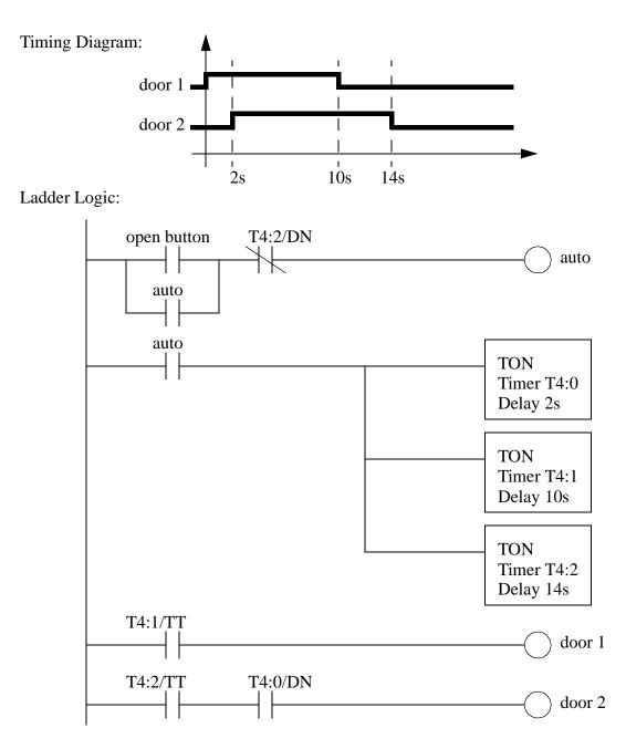
*Figure 10.5* Design With a Timing Diagram
