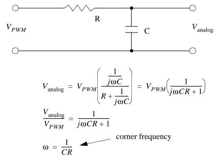
As an example consider that the PWM signal is used at a frequency of 100KHz, an it is to be used with a system that has a response time (time constant) of 0.1seconds. Therefore the corner frequency should be between 10Hz (1/0.1s) and 100KHz. This can be put at the mid point of 1000Hz, or 6.2Krad/s. This system also requires the arbitrary selection of a resistor or capacitor value. We will pick the capacitor value to be 0.1uF so that we don't need an electrolytic.
