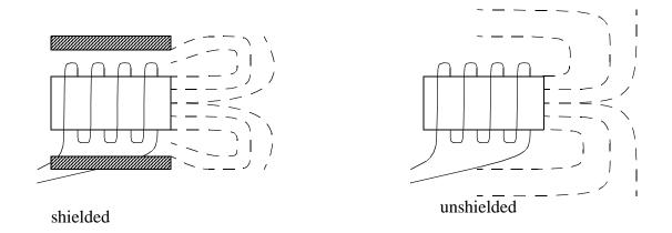
Figure 4.28 Shielded and Unshielded Sensors
