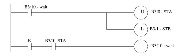
Figure 16.27 Subroutines for State STA to Prevent Racing
