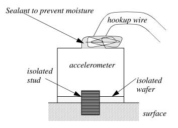
Figure 23.14 Mounting an Accelerometer
