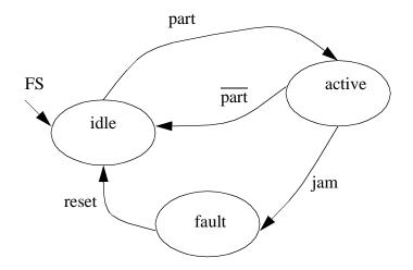
5. Use equations to develop ladder logic for the state diagram below using the delayed update method. Be sure to deal with the priority problems.
