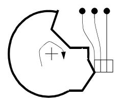
As the cam rotates it makes contact with none, one, or two terminals, as determined by the depressions and rises in the rotating cam.
