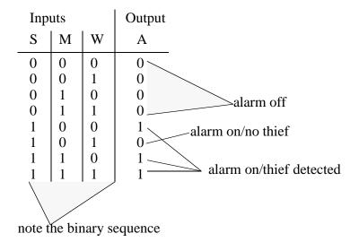
*Figure 6.20* Truth Table for the Alarm
