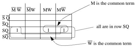
Step 5: Write the equation using the patterns
