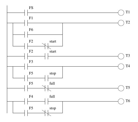
*Figure 11.11* The Transition Logic
