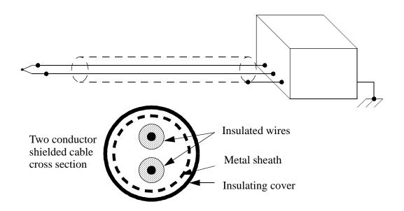
*Figure 22.17* Shielding for a Thermocouple
