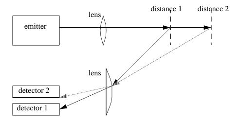
Figure 4.20 Multiple Point Detection Using Optics
