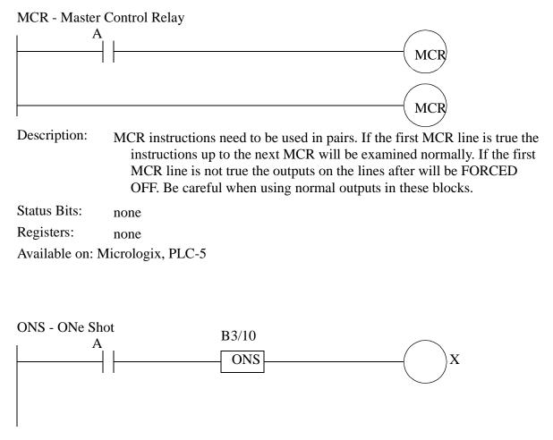
Description: This instruction will allow a line to be true for only one scan. If 'A' becomes true then output of the 'ONS' instruction will turn on for only one scan. 'A' must be turned off for one scan before the 'ONS' can be triggered again. The bit is used to track the previous input state, it is similar to an enabled bit.
