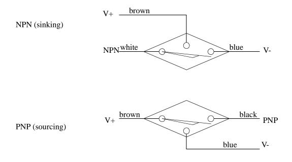
*Figure 4.9* Sourcing and Sinking Schematic Symbols
