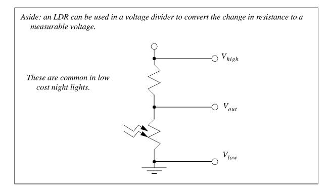
Figure 23.31 A Light Level Detector Circuit
