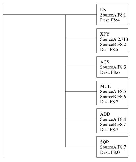
*Figure 15.7* An Equation in Ladder Logic
