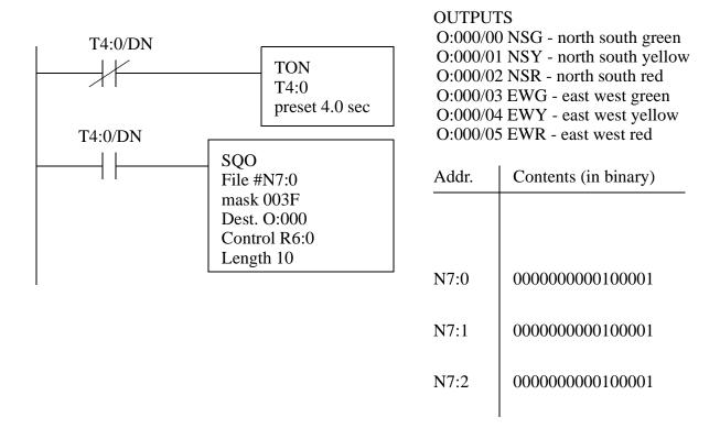
Figure 16.29 An Example Traffic Light Controller
