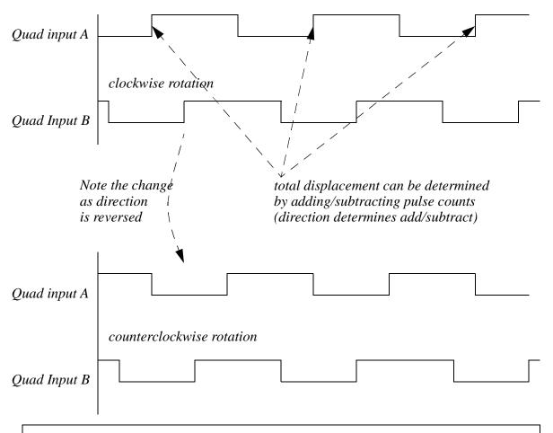
Note: To determine direction we can do a simple check. If both are off or on, the first to change state determines direction. Consider a point in the graphs above where both A and B are off. If A is the first input to turn on the encoder is rotating clockwise. If B is the first to turn on the rotation is counterclockwise.
