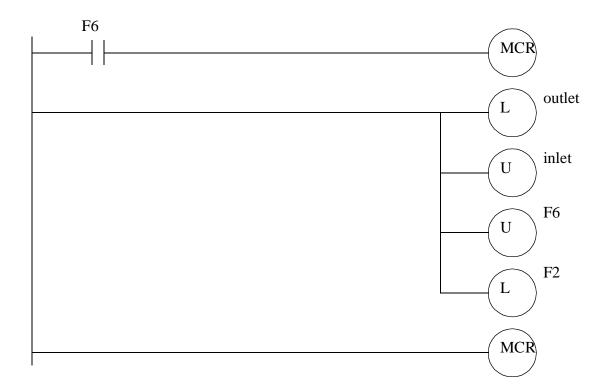
Figure 11.9 Ladder Logic for Operation F6
