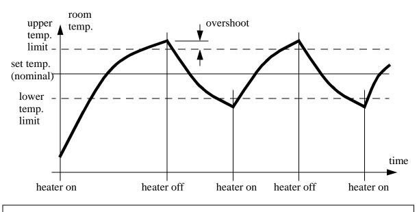
Note: This system turns on/off continuously. This behavior is known hunting. If the limits are set too close to the nominal value, the system will hunt at a faster rate. Therefore, to prevent wear and improve efficiency we normally try to set the limits as far away from nominal as possible.
