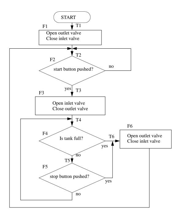
Figure 11.10 Label the Flowchart Blocks and Arrows
