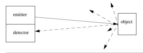
Note: with diffuse reflection the light is scattered. This reduces the quantity of light returned. As a result the light needs to be amplified using lenses.
