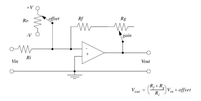
*Figure 23.34* A Single Ended Signal Amplifier
