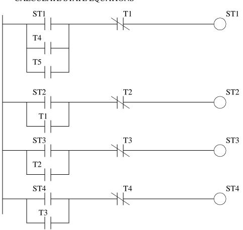
*Figure 12.29* Ladder Logic for the State-Transition Equations
