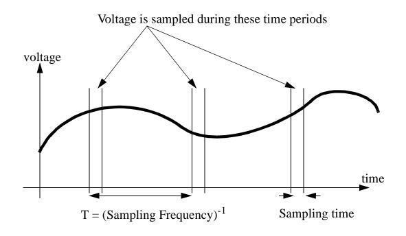
*Figure 22.2* Sampling an Analog Voltage
