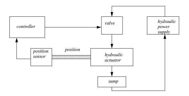
Figure 24.21 Hydraulic Servo System
