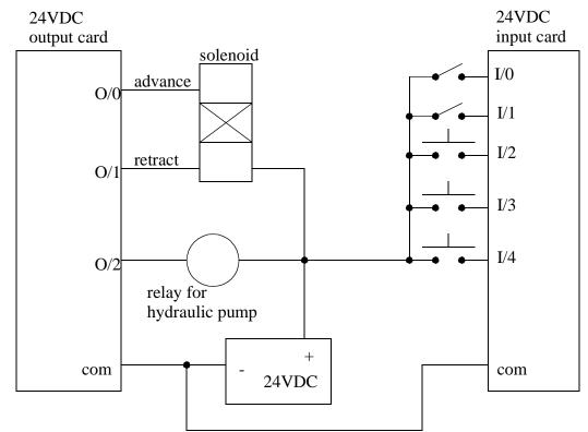
*Figure 3.8* Case Study for Press Wiring
