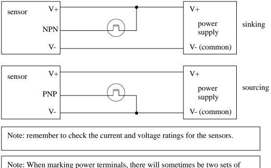
markings. The more standard is V+ and COM, but sometimes you will see devices and power supplies without a COM (common), in this case assume the V- is the common.
