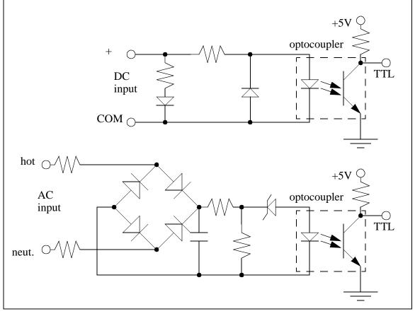
Figure 3.3 Aside: PLC Input Circuits
