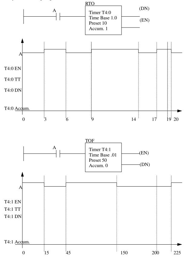
8. Complete the timing diagrams for the two timers below.
