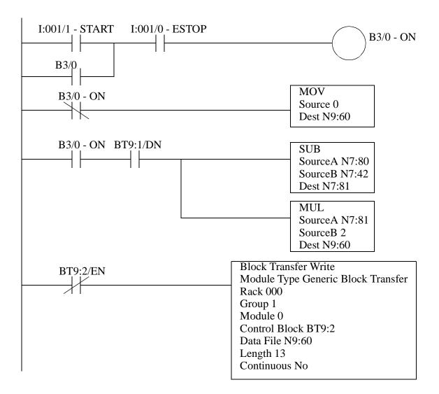
Figure 25.12 Implementing a Proportional Controller with Ladder Logic
