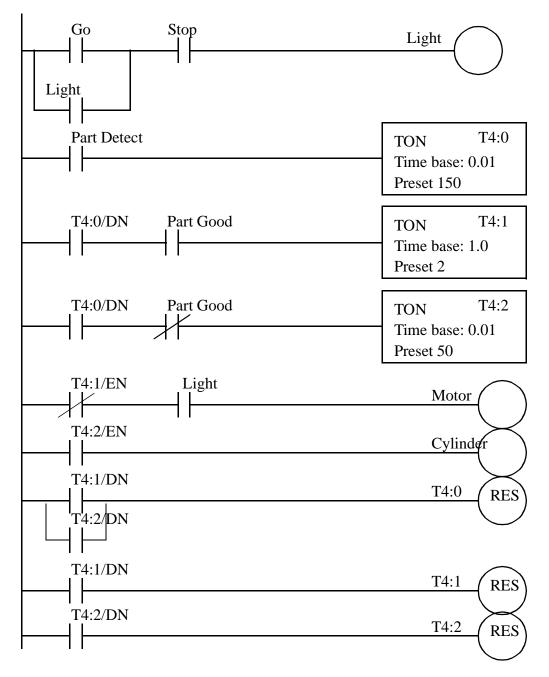
*Figure 9.26* A Conveyor Sorting Example
