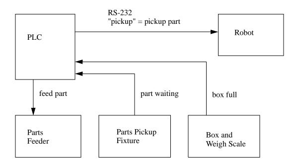
Figure 27.12 Box Loading System
