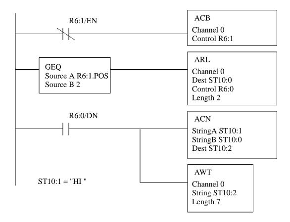
*Figure 27.9* An ASCII String Example
