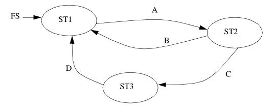
3. Convert the following state diagram to ladder logic using the block logic method. Give the stop button higher priority.
