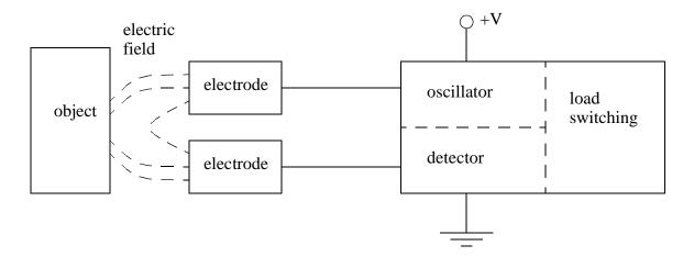
NOTE: For this sensor the proximity of any material near the electrodes will increase the capacitance. This will vary the magnitude of the oscillating signal and the detector will decide when this is great enough to determine proximity.
