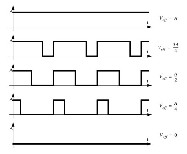
Figure 22.15 Pulse Width Modulated (PWM) Signals
