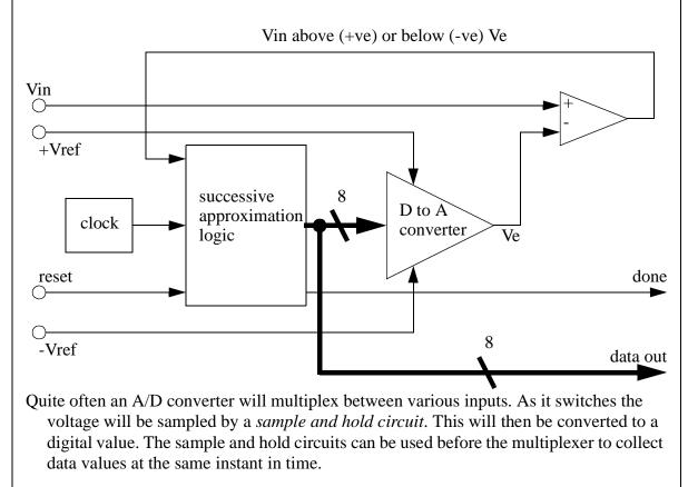
Figure 22.7 A Successive Approximation A/D Converter
