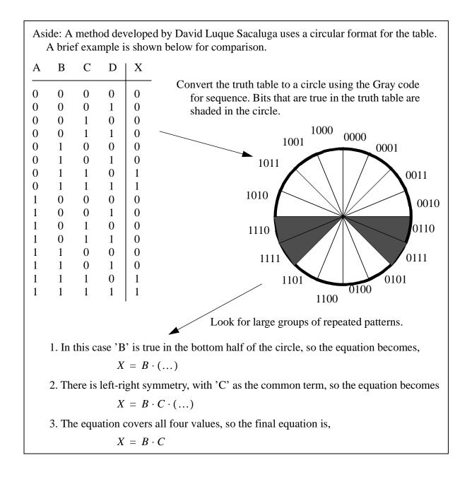
*Figure 7.4* Aside: An Alternate Approach
