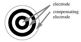
Note: the compensating electrode is used for negative feedback to make the sensor more resistant to variations, such as contaminations on the face of the sensor.
