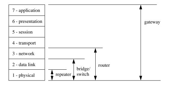
*Figure 28.4* Network Devices and the OSI Model
