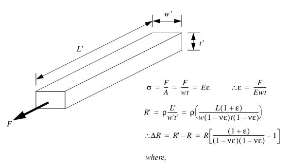
v = poissons ratio for the material F = applied force E = Youngs modulus for the material $\sigma, \varepsilon = stress and strain of material$
