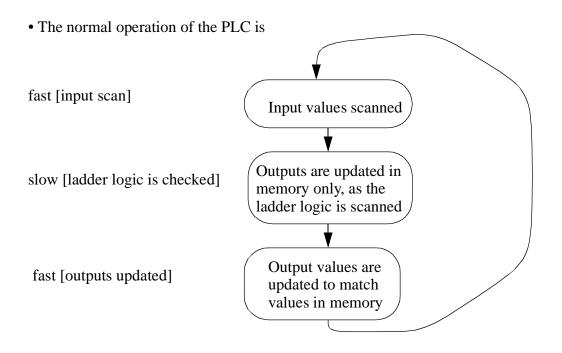
Figure 16.19 Input, Program and Output Scan
