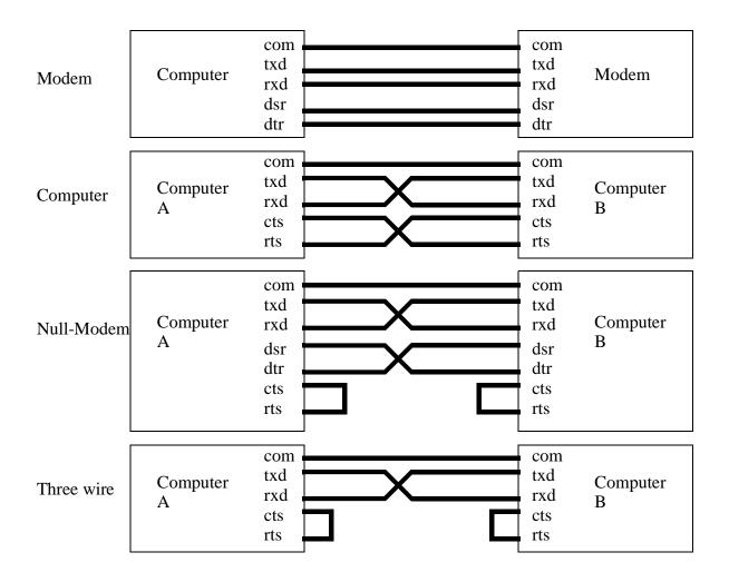
Figure 27.4 Common RS-232 Connection Schemes
