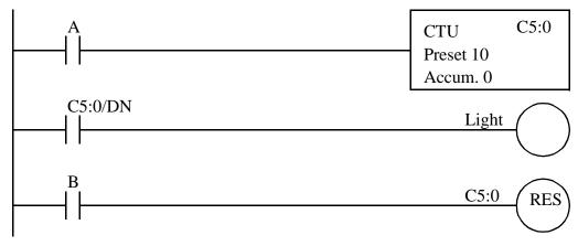
*Figure 9.22* A Simple Counter Example
