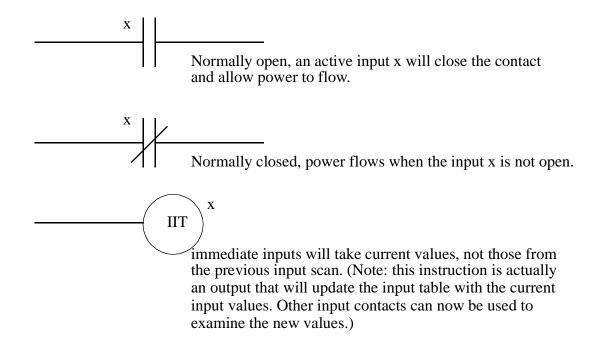
*Figure 2.11* Ladder Logic Inputs
