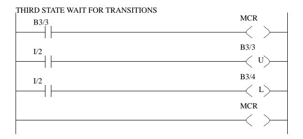
Figure 12.14 Ladder Logic for State Three
