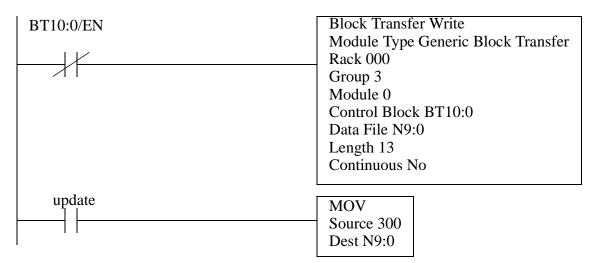
Figure 22.13 Controlling a 1771-OFE Analog Output Card
