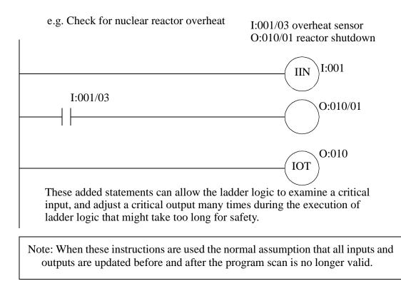
Figure 16.20 Immediate Inputs and Outputs
