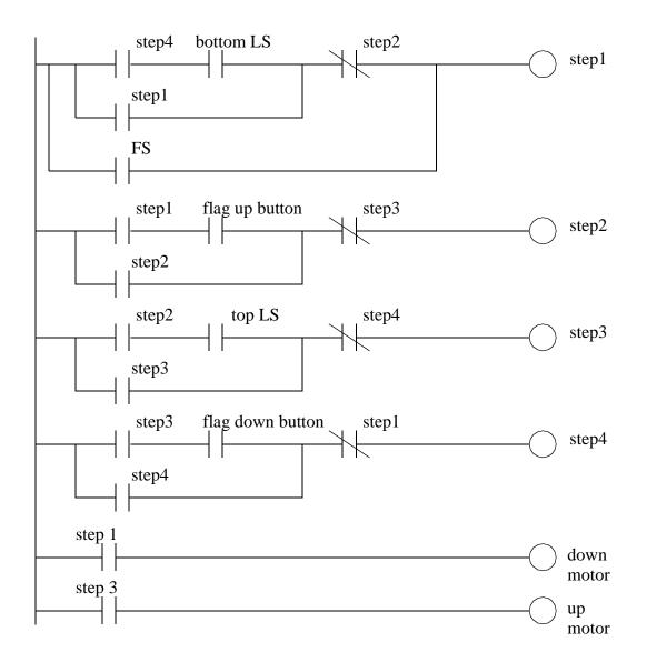
Figure 10.4 Process Sequence Bits Without Latches
