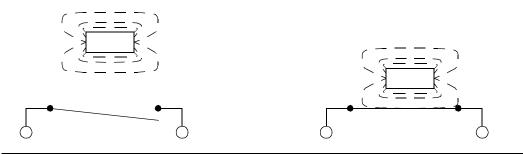
Note: With this device the magnet is moved towards the reed switch. As it gets closer the switch will close. This allows proximity detection without contact, but requires that a separate magnet be attached to a moving part.
