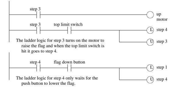
*Figure 10.3* A Process Sequence Bit Design Example (continued)
