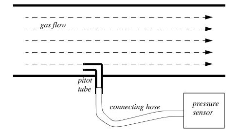
Figure 23.25 Pitot Tubes for Measuring Gas Flow Rates
