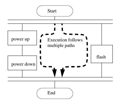
*Figure 2.7* An Example of a Sequential Function Chart
