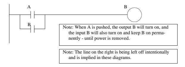
*Figure 2.4* A Seal-in Circuit
