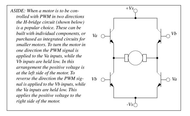
Figure 24.6 PWM Bidirectional Motor Control Circuit
