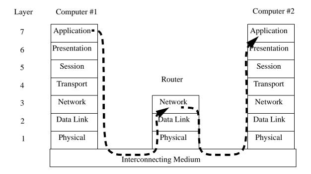
*Figure 28.5* The OSI Network Model with a Router
