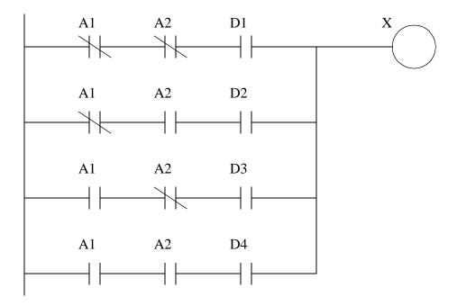
*Figure 6.14* A Multiplexer in Ladder Logic
