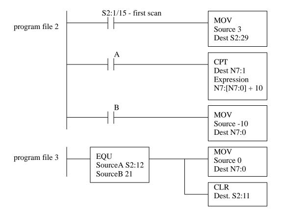
Figure 16.15 A Fault Recovery Program
