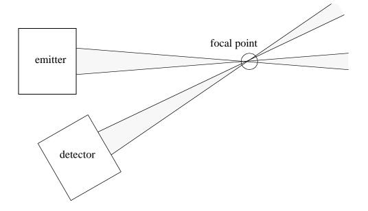
Figure 4.19 Point Detection Using Focused Optics
