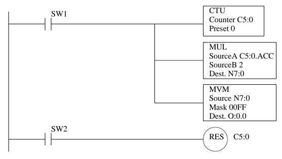
*Figure 15.24* A Simple Calculation Example
