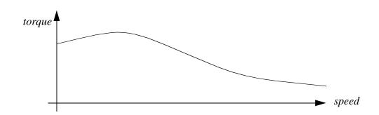
Figure 24.18 Stepper Motor Torque Speed Curve
