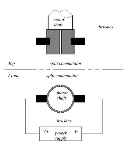
*Figure 24.3* A Split Ring Commutator
