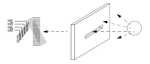
Figure 23.11 Measuring Motion with Moire Fringes
