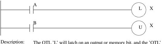
Description: The OTL 'L' will latch on an output or memory bit, and the 'OTL' 'U' will unlatch it. If a value has been changed with a latch its value will stay fixed even if the PLC has been restarted.
