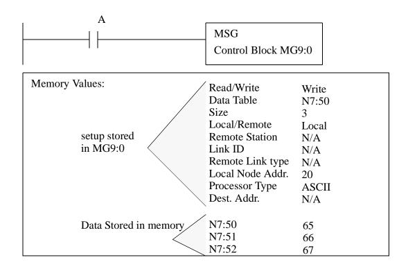
Figure 27.7 Message Function for Serial Communication
