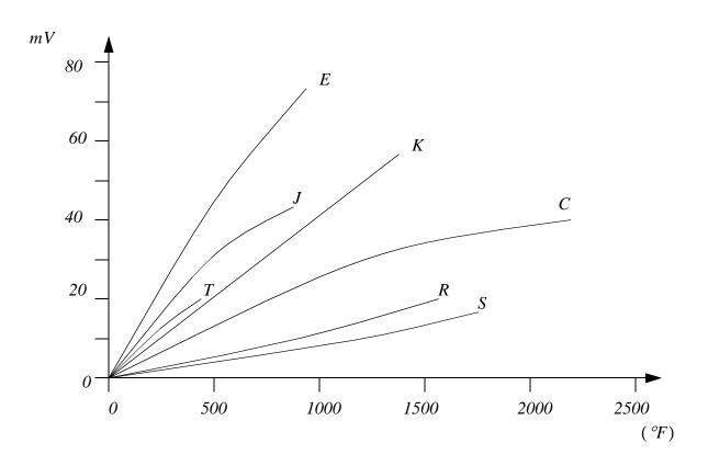
*Figure 23.28* Thermocouple Temperature Voltage Relationships (Approximate)
