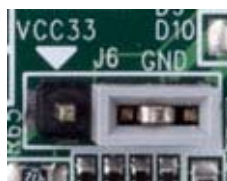
Figure 4. J6 Header Used for Selecting the JTAG Port of the PLDs
