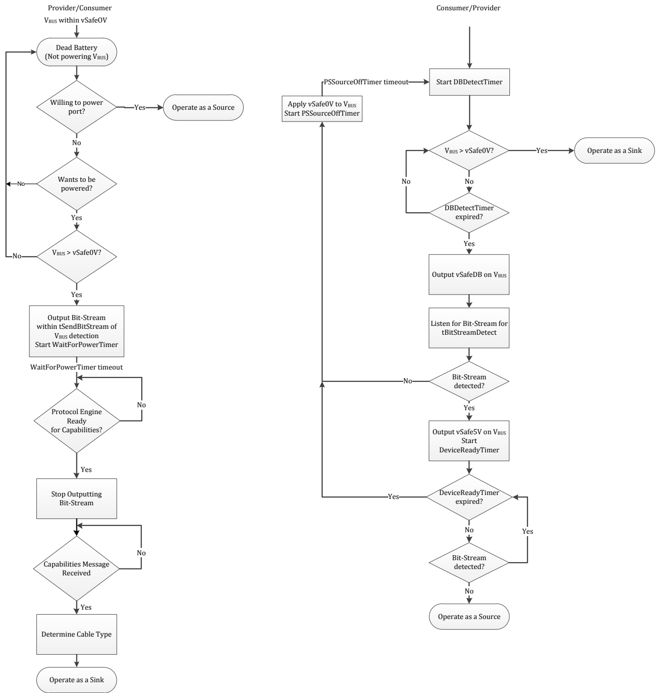
Figure 4-1 Dead Battery / Unpowered Port Detection Flow
