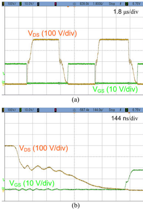
Fig. 13. (a) V_{GS} and V_{DS} of M_2 . (b) Detail of both voltages during the dead time.
