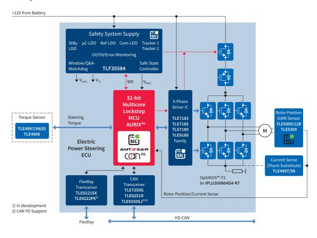
The new TriCore™ family AURIX™ with state-of-the-art safety features enables systems to achieve the highest safety level ASIL-D, which is already required in contemporary steering systems.
