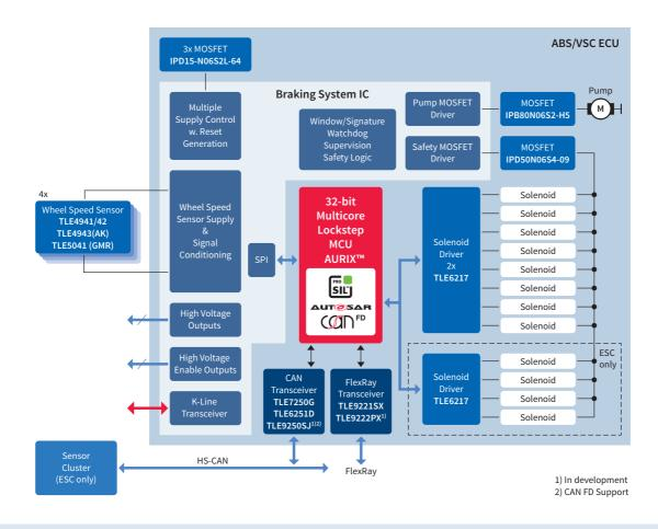
The new TriCore™ family AURIX™ with state-of-the-art safety features enables systems to achieve the highest safety level ASIL-D, which is already required in contemporary braking systems. The latest diverse lockstep technology with clock delay (Diverse Lockstep Core) reduces the software overhead significantly and enables fast time-to-market. The scalability supports an optimized cost-performance fit for basic ABS systems up to highly-integrated ESC systems.
