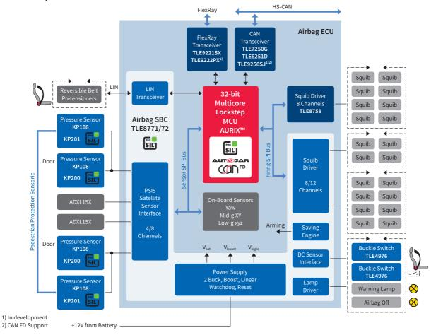
The new TriCore<sup>™</sup> family AURIX<sup>™</sup> with state-of-the-art safety features enables systems to achieve the highest safety level up to ASIL-D.
