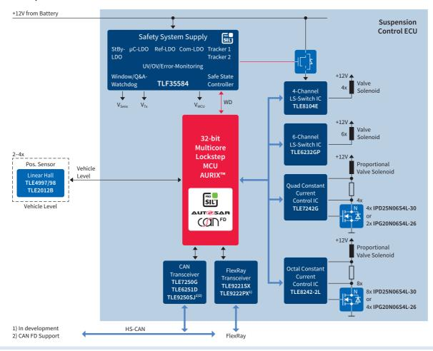
The new TriCore™ family AURIX™ with state-of-the-art safety features enables systems to achieve the highest safety level ASIL-D, which is already required in contemporary suspension systems.
