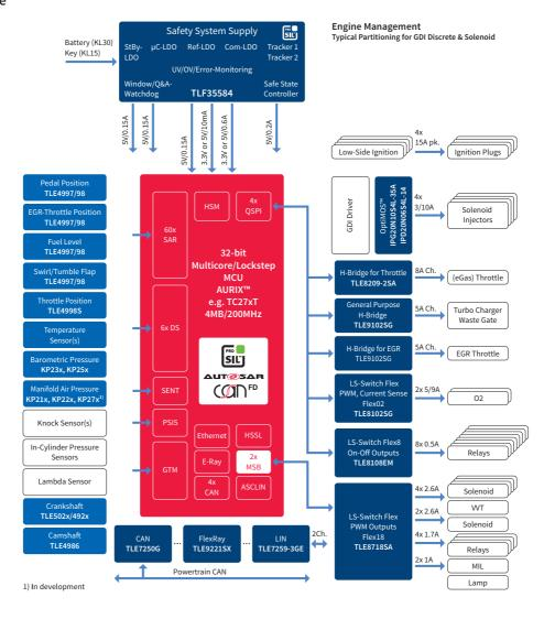
The new TriCore™ family AURIX™ with state-of-the-art safety features enables systems to achieve the highest safety level up to ASIL-D. The scalable AURIX™ family includes the GTM, the de-facto industry standard timing module that supports highly complex engine management, while meeting the market's most stringent emissions regulations.
