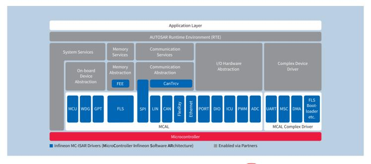
MC-ISAR MicroController – Infineon Software ARchitecture MC-ISAR: MCU, WDG, GPT, SPI, PORT, DIO, ICU, PWM, ADC
