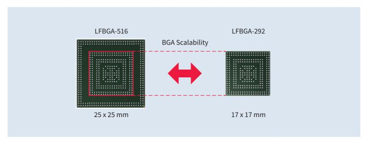
■ LFBGA-292 and LFBGA-516 are ball compatible so that customers can build one PCB for both packages
