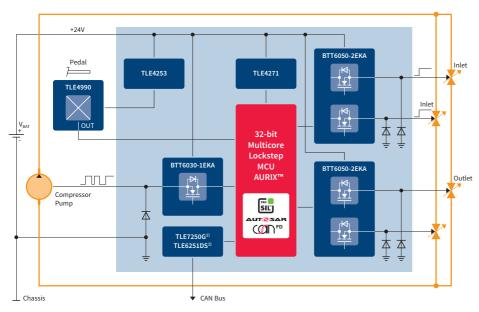
1) If ECU permanently supplied, you may need to add external protection against load dump 400ms above 40V  $\,$
