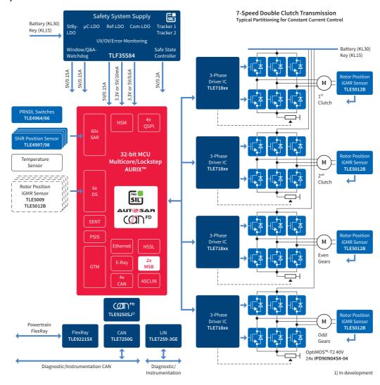
The new TriCore™ family AURIX™ with state-of-the-art safety features enables systems to achieve the highest safety level up to ASIL-D. The rich scalability of the AURIX™ family permits a platform approach that meets the needs of a range of transmission system demands. Furthermore, the hot temperature package and bare die solutions enable AURIX™ to be used in both attached and integrated control units.
