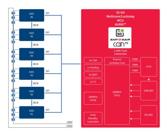
The battery management system controls the battery state during charging and discharging. Intelligent functionality is needed to extend the battery lifetime, which has a considerable impact on the total cost of ownership. The State of Health (SoH), State of Charge (SoC) and Depth of Discharge (DoD) of the battery is permanently monitored.
