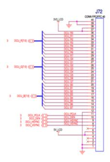
Figure 6. Typical connection to a TFT display using RGB bus
