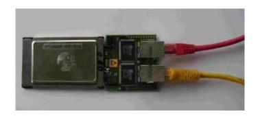
PRP is here handled by the main processor. Co-processor or FPGA can execute PRP as well.
