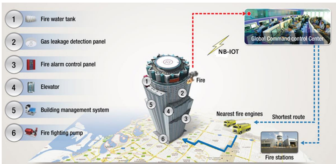
Figure 9: Alarm & Event Detectors
