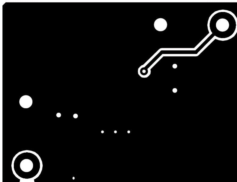
Figure 65. Bottom Layer of Example Converter Layout
