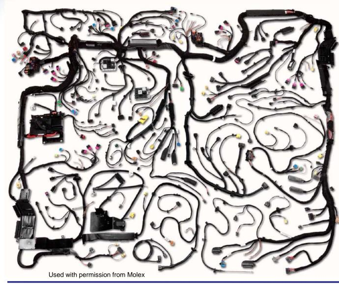
Cabling is the 3<sup>rd</sup> highest cost component in a car Engine (1st) Chassis (2nd)
