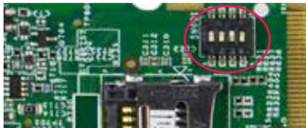
Figure 3. SW601 setting for internal boot mode
