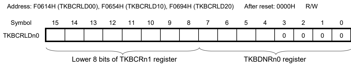
Figure 7-14. Format of 16-bit Timer KB Compare 1L & Dithering Count Register n0 (TKBCRLDn0)
