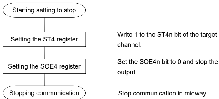
Figure 16-53. Procedure for Stopping DALI Transmission
