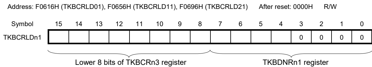
Figure 7-15. Format of 16-bit Timer KB Compare 3L & Dithering Count Register n1 (TKBCRLDn1)
