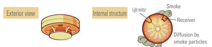
■ Figure 3 Photoelectric Spot Sensor
