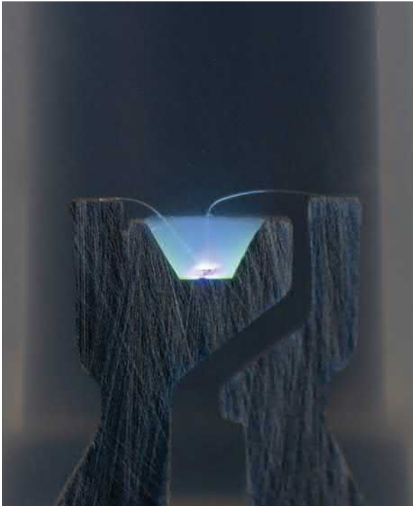
This image, a composite of photos with different exposure levels, reveals a hard-to-capture blue glow around the LED die.
