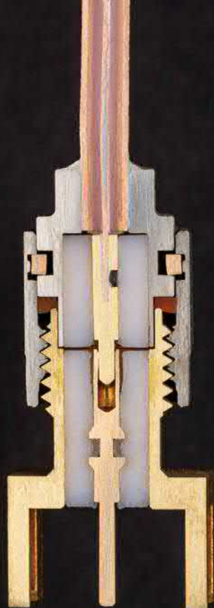
A tiny hole in the side of the plug's center pin is for soldering that pin to the center conductor of the semi-rigid coax: molten solder flows into the junction and securely fastens the two pieces of metal together.
