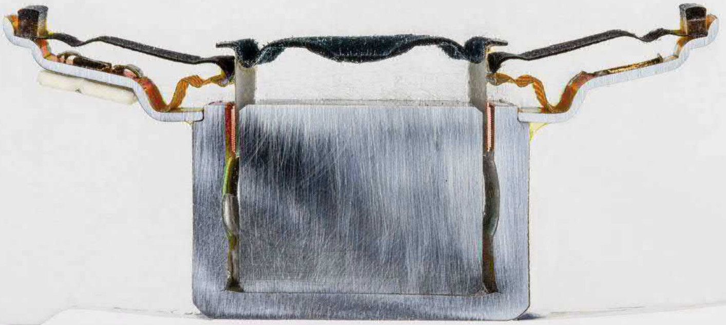
This thin slice through a speaker was cast in transparent resin.
