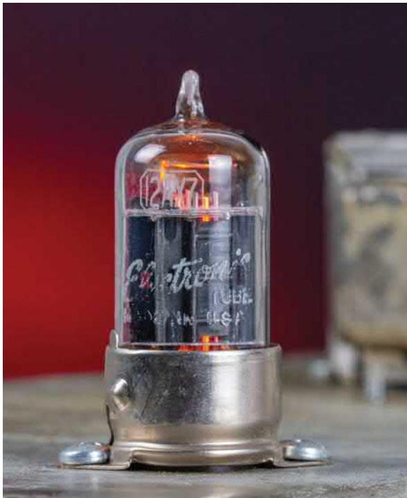
The vacuum in the tube allows the electrons to flow freely, without interacting with air molecules.
