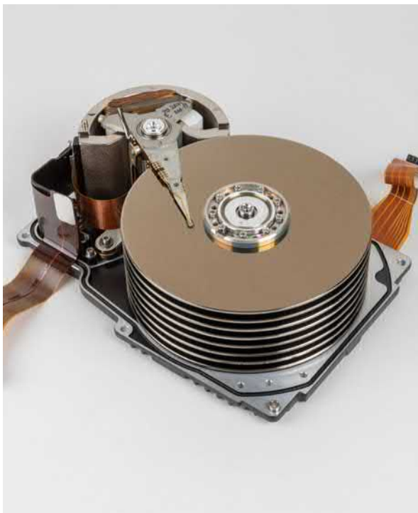
This 2 GB Micropolis-brand hard drive from 1992 has eight platters for storing data.
