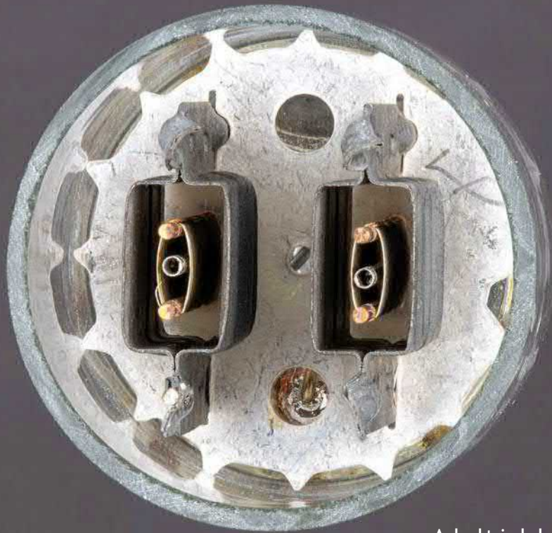
A dual triode has two copies of the main structure within.
