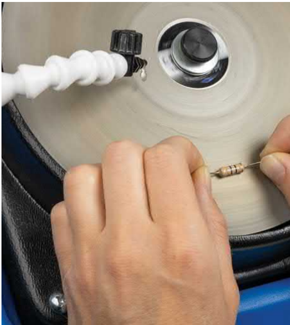
A diamond-coated disc cuts through the ceramic core of a carbon film resistor.
