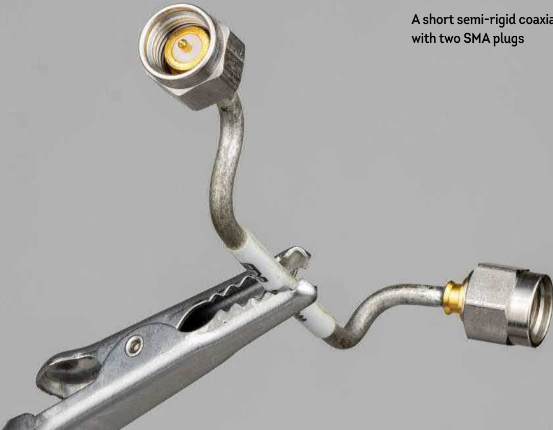
A tiny hole in the side of the plug's center pin is for soldering that pin to the center conductor of the semi-rigid coax: molten solder flows into the junction and securely fastens the two pieces of metal together.
