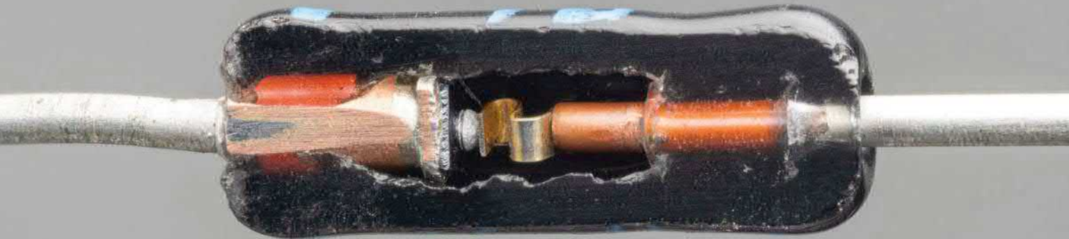
The clear glass has been painted black on the outside of this 1N5236B Zener diode. An S-shaped spring makes contact with the die.
