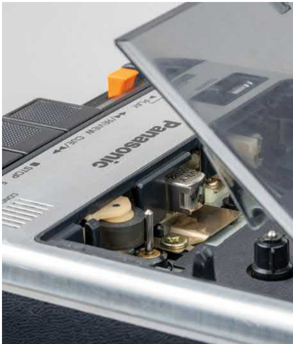
Two tape heads are visible in a Panasonic-brand cassette tape recorder. The metal one in the center is for playback and recording. The white plastic head beside it is for erasing a preexisting recording.
