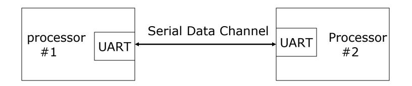
In most computer systems, the UART is connected to circuitry that generates signals that comply with the EIA (Electronics Industries Association) RS232-C specification.
