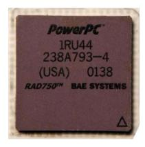
Based on re-engineered commercial technology, it is a licensed, rad-hard version of the IBM PowerPC 750. With nearly 10 times the performance of current rad-hard space processors, the RAD750 processor is the most powerful radiation-hardened general-purpose microprocessor ever developed.
