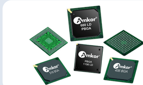
Figure 1. Flip Chip Package Outline (FCBGA). (Source: Amkor Technology Inc. ©2025)
