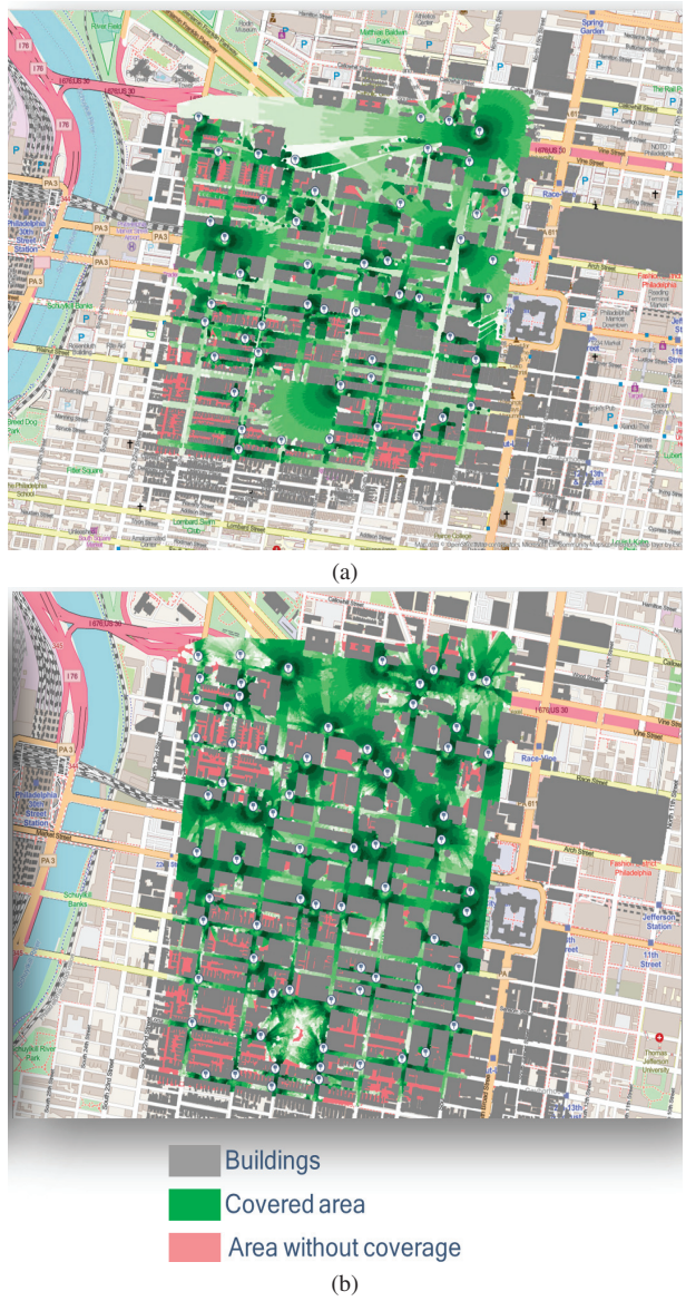
Figure 5.15 SNR coverage map when foliage (a) is not accounted for and (b) is accounted for. Map data from OpenStreetMap with license agreement covering this usage available at https://www.openstreetmap.org/copyright .
