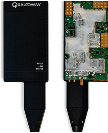
Figure 3.11 Prototype UE with multiple 4 \times 2 arrays on the front and back faces.
