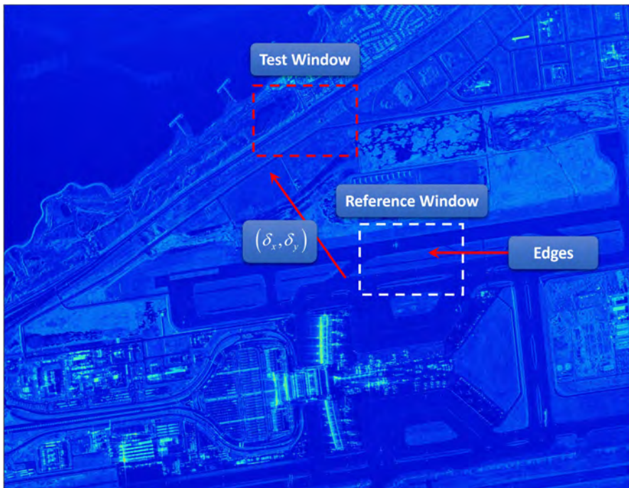
Figure 6.6 Reference and test windows in an edge region. SAR imagery of Muscat International Airport in Oman. Courtesy of ICEYE.
