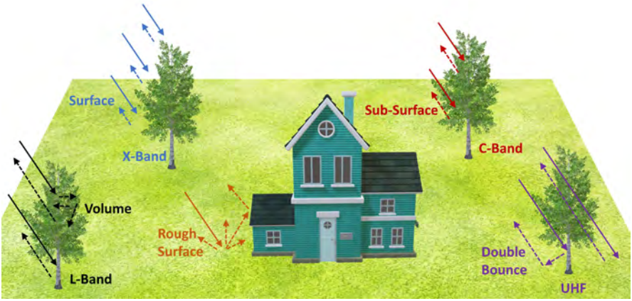
Figure 1.4 Scattering mechanisms and penetration by frequency band.
