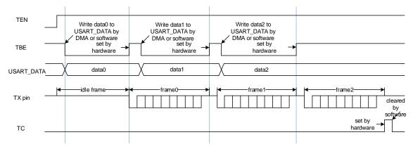
It is necessary to wait for the TC bit asserted before disabling the USART or entering the power saving mode. This bit can be cleared by a software sequence: reading the USART\_STAT register and then writing the USART\_DATA register. If the multibuffer communication is selected (DENT=1), this bit can also be cleared by writing 0 to it directly.
