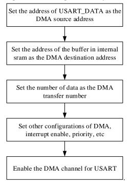
When the number of the data received by USART reaches the DMA transfer number, an end of transfer interrupt can be generated in the DMA module.
