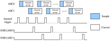
If the discontinuous mode is enabled for both ADC0 and ADC1, when the first trigger occurs, the first inserted channel in ADC0 is converted. When the second trigger occurs, the first inserted channel in ADC1 is converted. Then the second channel in ADC0, the second channel in ADC1, and so on.
