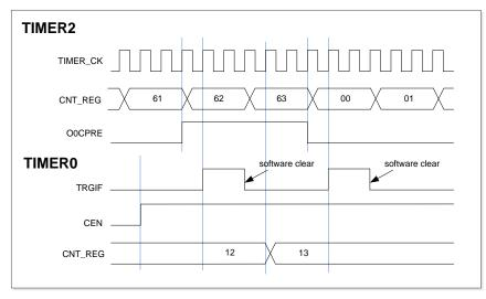
Using an external trigger to start 2 timers synchronously
