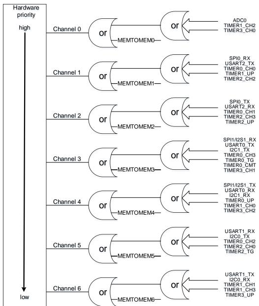
Figure 9-4. DMA0 request mapping
