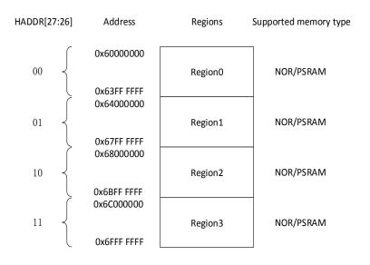
HADDR[25:0] is the byte address whereas the external memory may not be byte accessed, this will lead to address inconsistency. EXMC can adjust HADDR to accommodate the data width of the external memory according to the following rules.
