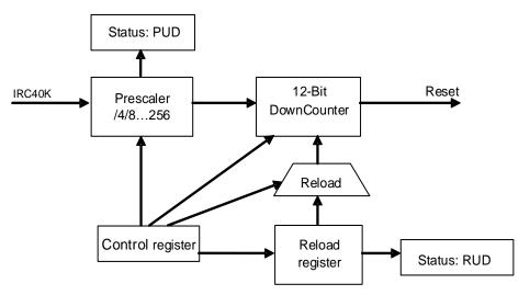
The free watchdog is enabled by writing the value 0xCCCC in the control register (FWDGT\_CTL), and the counter starts counting down. When the counter reaches the value 0x000, a reset is generated.
