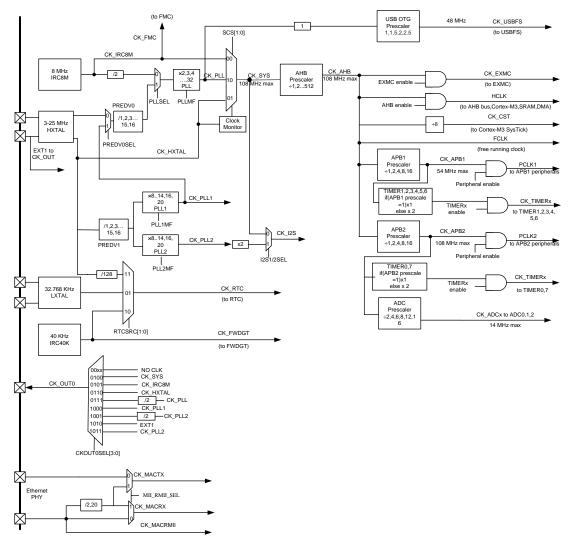
The frequency of AHB, APB2 and the APB1 domains can be configured by each prescaler. The maximum frequency of the AHB, APB2 and APB1 domains is 108 MHz/108 MHz/54 MHz. The Cortex System Timer (SysTick) external clock is clocked with the AHB clock (HCLK) divided by 8. The SysTick can work either with this clock or with the AHB clock (HCLK), configurable in the SysTick Control and Status Register.
