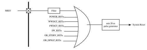
Figure 5-4. The system reset circuit
