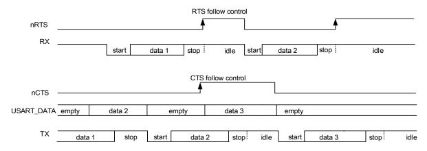
If the CTS flow control is enabled, the CTSF bit in USART\_STAT is set when the nCTS pin toggles. An interrupt is generated if the CTSIE bit in USART\_CTL2 is set.
