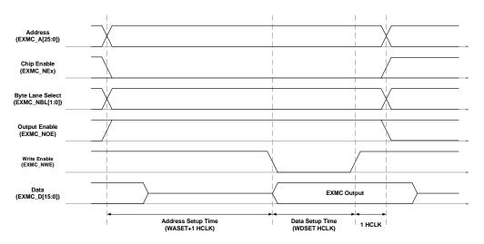
The different between mode A and mode 1 write timing is that read/write timing is specified by the same set of timing configuration, while mode A write timing configuration is independent of its read configuration.
