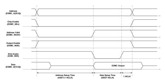
Figure 20-12. Mode B write access
