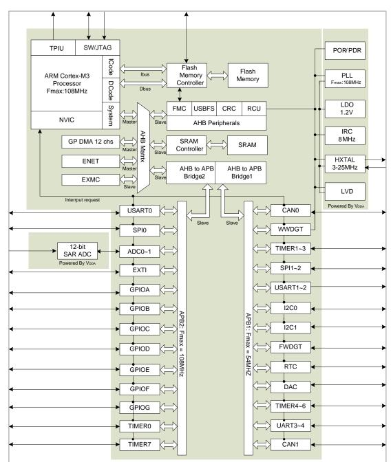
Figure 1-5. GD32F10x Connectivity line series system architecture
