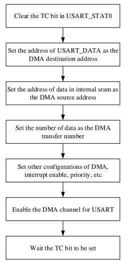
After all of the data frames are transmitted, the TC bit in USART\_STAT is set. An interrupt occurs if the TCIE bit in USART\_CTL0 is set.
