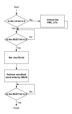
For the GD32F10x\_CL and GD32F10x\_XD, the program procedure applied to bank1 is similar to the procedure applied to bank0.
