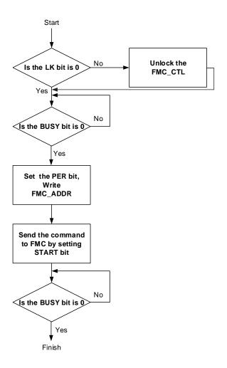
For the GD32F10x\_CL and GD32F10x\_XD, FMC\_STAT0 reflects the operation status of bank0, and FMC\_ STAT1 reflects the operation status of bank1. The page erase procedure applied to bank1 is similar to the procedure applied to bank0. Especially, when erasing page in bank1 under security protection, the address should not only be written to FMC\_ADRR1 but also to FMC\_ADDR0.
