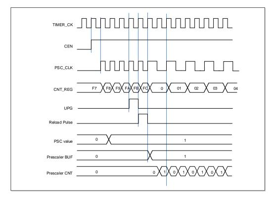
Figure 15-78. Counter timing diagram with prescaler division change from 1 to 2
