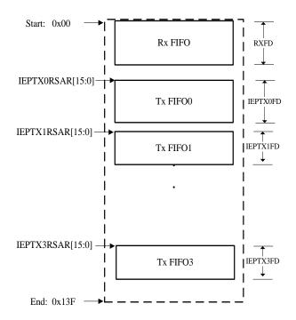
USBFS provides a special register area for the internal data FIFO reading and writing. *Figure* **24-8.** *Device mode FIFO access register map* describes the register memory area where the data FIFO can write. This area can be read by any endpoint FIFO. The addresses in the figure are addressed in bytes. Each endpoint has its own FIFO access register space. Rx FIFO is also able to be accessed using USBFS\_GRSTATR/USBFS\_GRSTATP register.
