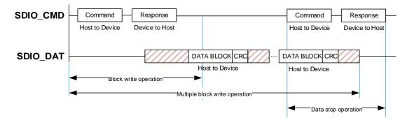
Data transfers to/from SD memory cards, SD I/O cards (both IO only card and combo card) and CE-ATA device are done in data blocks. Data transfers to/from MMC are done in data blocks or streams. *Figure 19-4. SDIO sequential read operation* and *Figure 19-5. SDIO sequential write operation* are the stream read and write operation.
