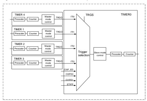
Figure 15-26. Timer0 master/slave mode timer example
