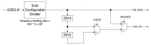
The block diagram of I2S clock generator is shown as *Figure 18-44. Block diagram of I2S clock generator*. The I2S interface clocks are configured by the DIV bits, the OF bit, the
