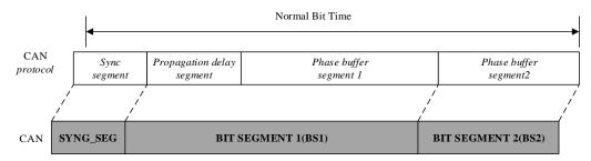
The resynchronization Jump Width (SJW) defines an upper bound to the amount of lengthening or shortening of the bit segments. It is programmable between 1 and 4 time quanta.
