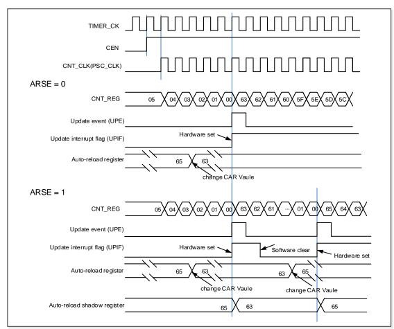
Figure 15-72. Down-counter timechart, change TIMERx\_CAR on the go
