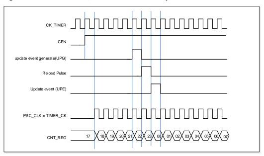
Figure 15-77. Normal mode, internal clock divided by 1
