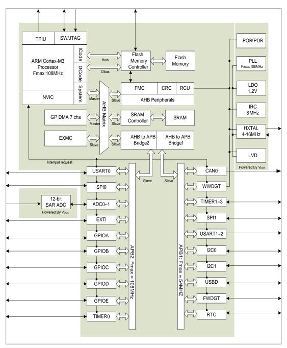
Figure 1-2. GD32F10x Medium-density series system architecture
