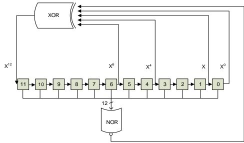
Figure 12-2. DAC LFSR algorithm
