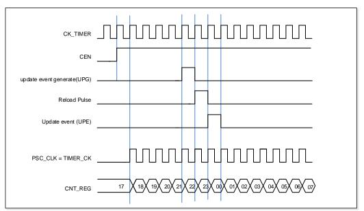
Figure 15-67. Normal mode, internal clock divided by 1
