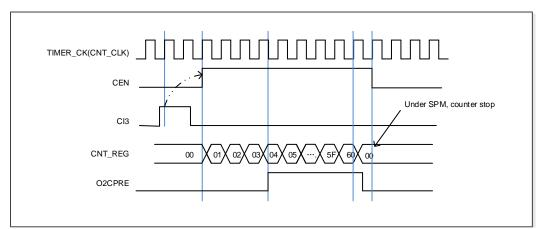
Figure 15-25. Single pulse mode, TIMERx\_CHxCV = 0x04, TIMERx\_CAR=0x60
