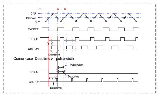
Figure 15-16. Complementary output with dead-time insertion
