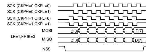
In normal mode, the length of data is configured by the FF16 bit in the SPI\_CTL0 register. Data length is 16 bits if FF16=1, otherwise is 8 bits.
