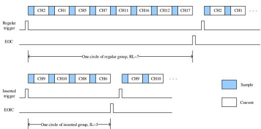
Software procedure for scan conversion on a regular channel group:
