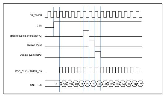
Figure 15-51. Normal mode, internal clock divided by 1
