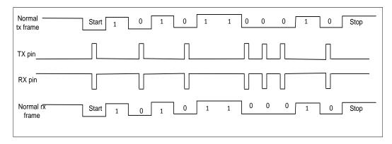
The SIR submodule can work in low power mode by setting the IRLP bit in USART\_CTL2. The transmit encoder is driven by a low speed clock, which is divided from the PCLK. The divide ratio is configured by the PSC[7:0] bits in USART\_GP register. The pulse width on the TX pin is 3 cycles of this low speed clock. The receiver decoder works in the same manner as the normal IrDA mode.
