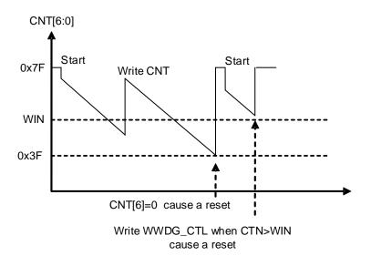
Calculate the WWDGT timeout by using the formula below.
