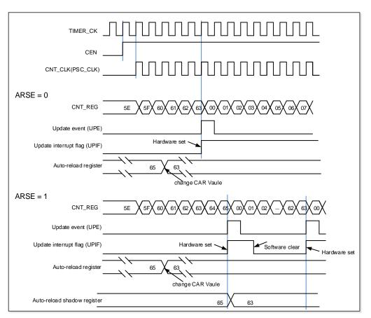
Figure 15-36. Up-counter timechart, change TIMERx\_CAR on the go.
