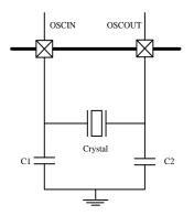
The HXTAL crystal oscillator can be switched on or off using the HXTALEN bit in the Control Register RCU\_CTL. The HXTALSTB flag in Control Register RCU\_CTL indicates if the high-speed external crystal oscillator is stable. When the HXTAL is powered up, it will not be released for use until this HXTALSTB bit is set by the hardware. This specific delay period is known as the oscillator "Start-up time". As the HXTAL becomes stable, an interrupt will be
