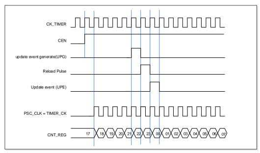
Figure 15-2. Normal mode, internal clock divided by 1
