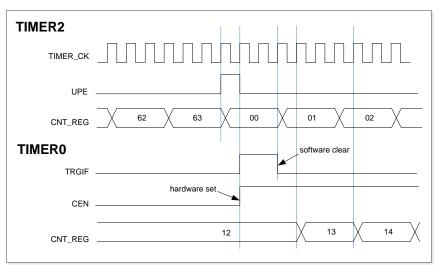
■ Enable Timer0 count with Timer2's enable/O0CPRE signal
