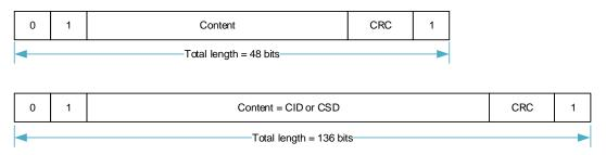
A response always starts with a start bit (always 0), followed by the bit indicating the direction of transmission (card = 0). A value 'x' in the tables below indicates a variable entry. All responses except for the type R3 are protected by a CRC. Every command code word is terminated by the end bit (always 1).
