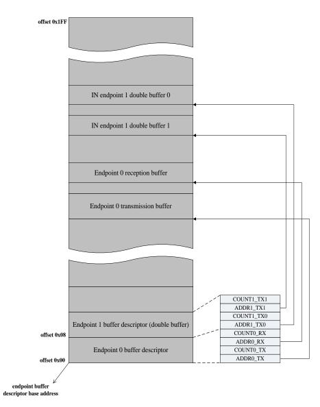
**Note:** This figure is not drawn on the actual scale, and it is addressed through the USB bus 16-bit mode.
