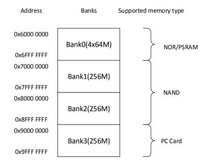
EXMC access space is divided into multiple banks. Each bank is 256 Mbytes. The first bank (Bank0) is further divided into four Regions, and each Region is 64 Mbytes. Bank1 and bank2 is each divided into two spaces, the attribute memory space and the common memory space. Bank3 is divided into three spaces, which are the attribute memory space, the common memory space and the I/O memory space.
