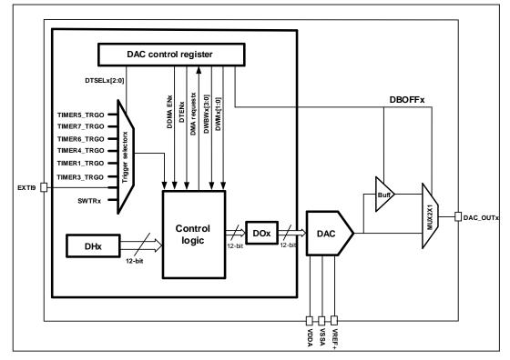
**Note:** In connectivity line devices, the TIMER7\_TRGO trigger is replaced by TIMER2\_TRGO.
