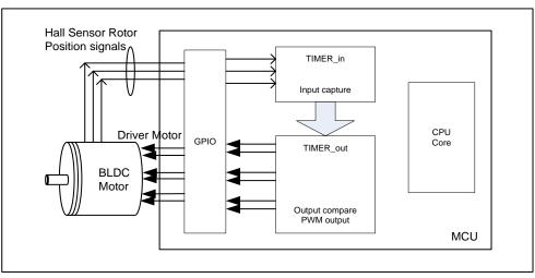
Figure 15-21. Hall sensor timing between two timers
