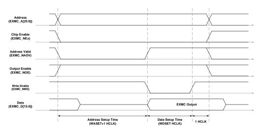
The different between mode C and mode 1 write timing is that read/write timing is specified by the same set of timing configuration, while mode C write timing configuration is independent of its read configuration.
