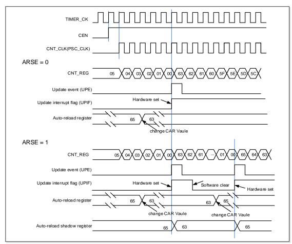
Figure 15-7. Down-counter timechart, change TIMERx\_CAR on the go
