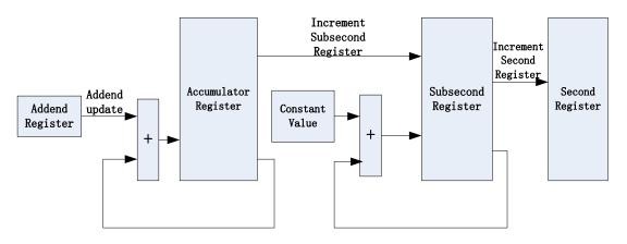
The following concrete example is used to descript the fine correction method how to update the system time:
