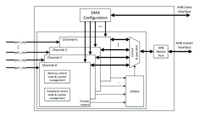
As shown in *Figure 9-1. Block diagram of DMA*, a DMA controller consists of four main parts:
