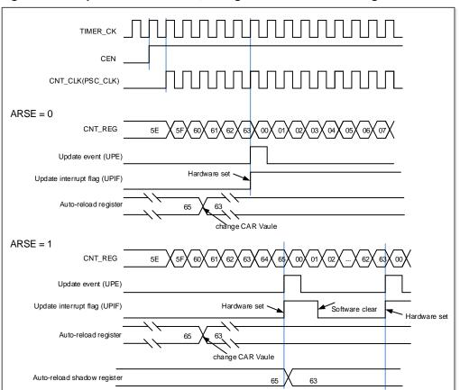
Figure 15-70. Up-counter timechart, change TIMERx\_CAR on the go
