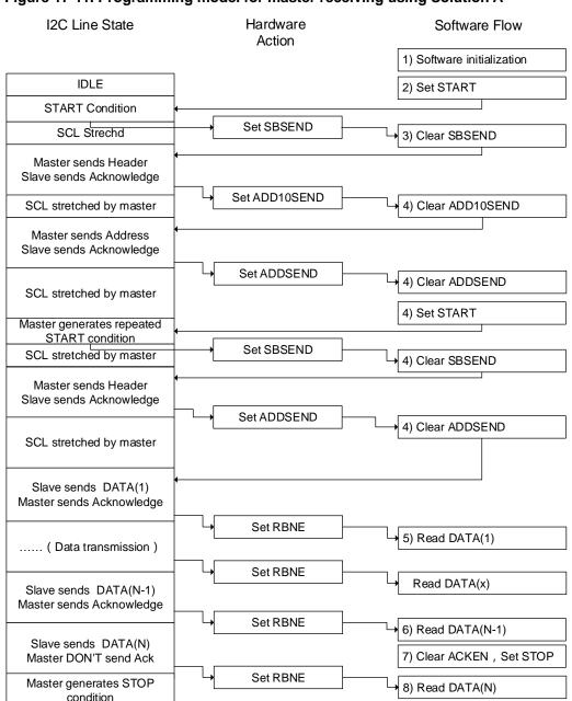
Figure 17-11. Programming model for master receiving using Solution A
