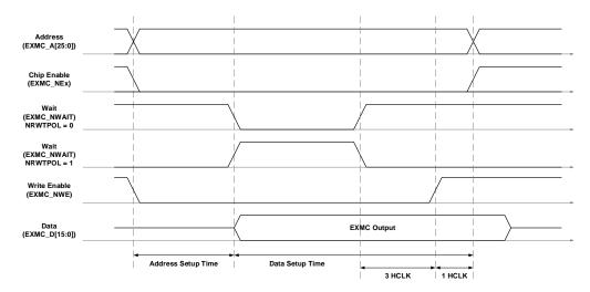
Figure 20-20. Write access timing diagram under async-wait signal assertion
