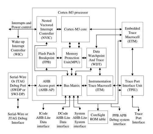
Figure 1-1. The structure of the Cortex<sup>™</sup>-M3 processor
