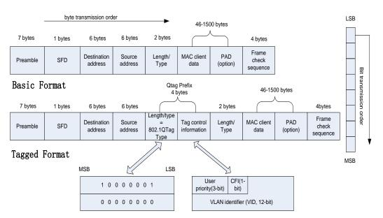
**Note:** The Ethernet controller transmits each byte at LSB first except FCS field.
