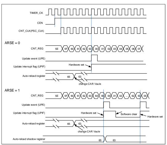
Figure 15-5. Up-counter timechart, change TIMERx\_CAR on the go
